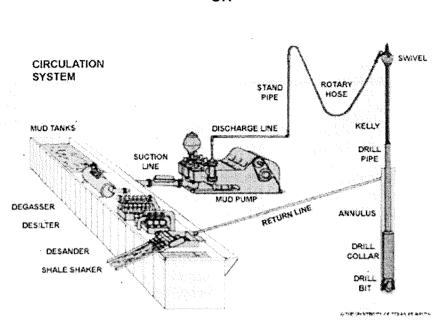
Drilling mud is a important part for the drilling work to maintain the wellbore; Cool, lubricate and support the bit and drilling and so on and most important remove cuttings well. Then here it problem, to reuse the drilling mud. Then it is the time for mud circulating system to come here.
