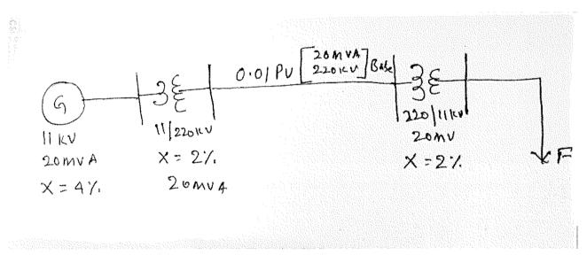
It is considered that a 3phase to ground symmetrical solid fault occurs at the secondary side of the transformer –T2.[ at point F]
