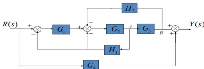
10. a. The robot arms used in industrial manufacturing require control of the position of the end piece. The simplified block diagram model of the system is shown below and has parameters  $\zeta = 0.6$  and  $\omega_n = 5 \text{ rad/sec}$ . The system is subjected to a unit step input. Estimate all the possible time response specification and comment on its performance
