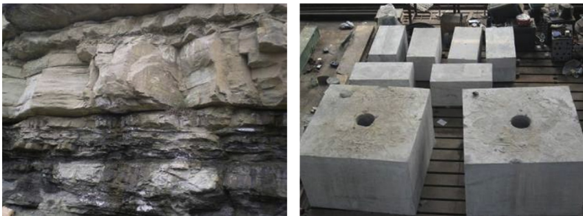
Figure 2.14 Sampling location and completed rock sample of Chang 6 stratum.
