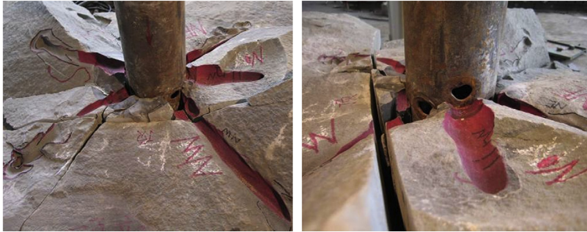
Figure 2.22 Dissected process of the No. 9 test assembly with rock sample.
