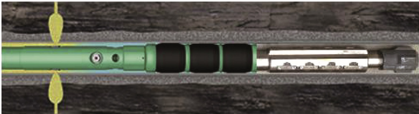
Figure 8.8 Hydra-jet perforating, annular path pumping working process.
