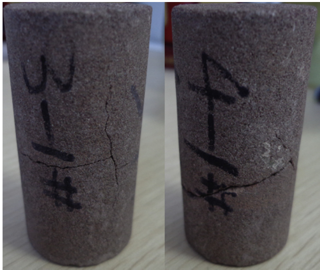
Figure 9.23 Sandstone samples after liquid nitrogen cooling.
