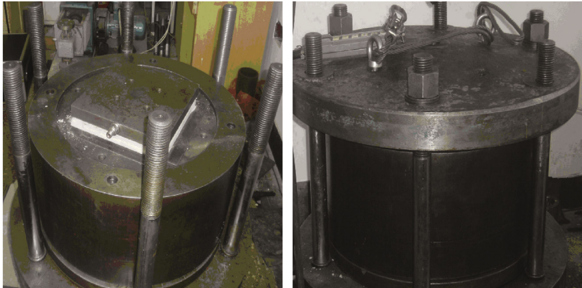
Figure 4.17 Picture of the true triaxial simulator.
