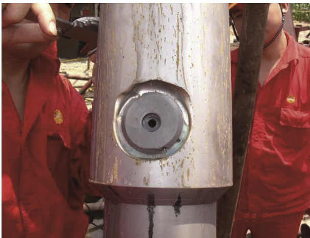
Figure 8.5 Used tool in Well BQ-110.
