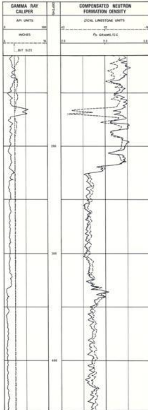
Figure 7.3. Example of Gamma Ray, Formation Density, and Compensated Neutron Logs in a limestone-dolomite succession (after Schlumberger).
