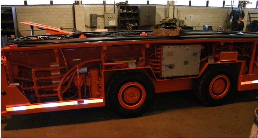
Figure 9.2 The auxiliary unit for in-mine horizontal drilling.
