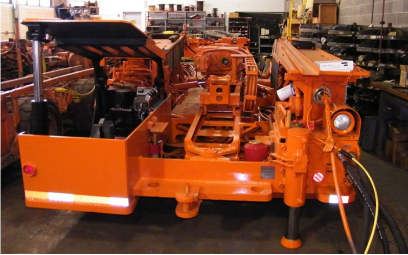
Figure 9.1 The drill unit for in-mine horizontal drilling.
