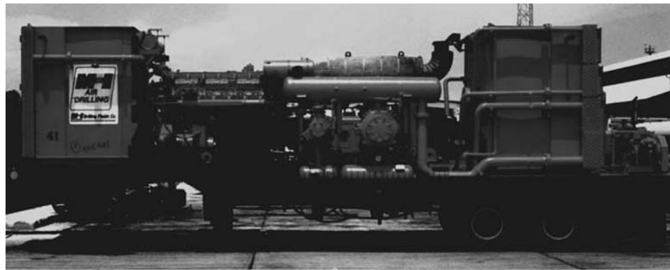
FIGURE 5-20. Semitrailer-mounted, four-stage reciprocating piston compressor system unit (courtesy of Air Comp Drilling).
