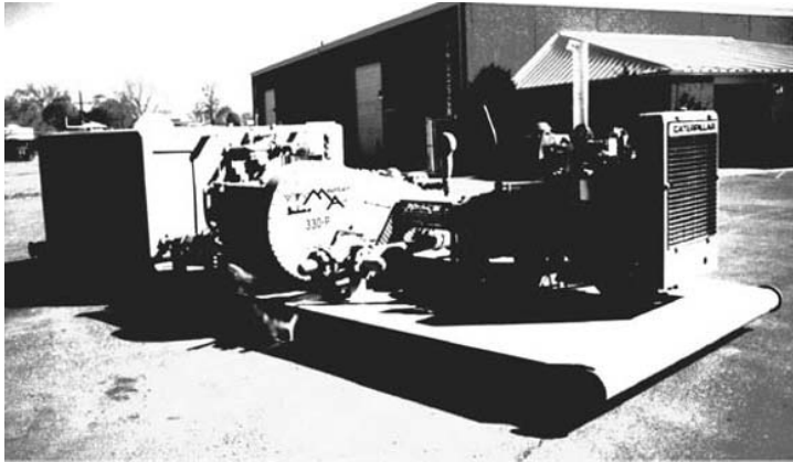
FIGURE 3-2. Water injection pump (courtesy of Mountain Air Drilling Services).
