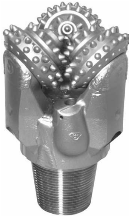
FIGURE 2-1. Tungsten carbide insert 7 7/8 inch (200.1 mm) tricone roller cutter bit IADC Code 627 (courtesy of Hughes Christensen Incorporated).
