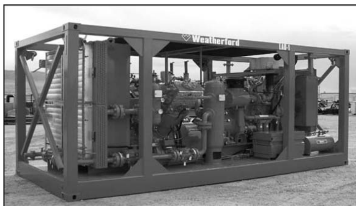
FIGURE 5-23. Skid-mounted, reciprocating piston high pressure booster compressor system unit (courtesy of Weatherford International).
