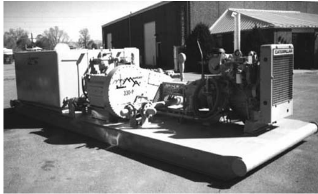
FIGURE 8-10. Liquid “mist” pump for air (or membrane generated nitrogen) drilling operations.
