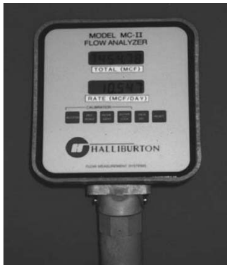
FIGURE 3-6. Digital display for the turbine flowmeter (courtesy of Halliburton Energy Services, Incorporated).
