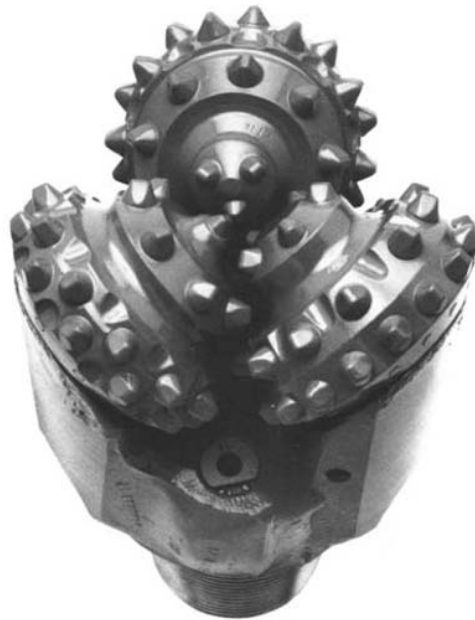
FIGURE 4-8. Insert tooth 7 7/8-in (200 mm)-diameter tricone roller cutter bit IADC Code 517 (courtesy of Reed Rock Bit Company).
