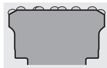
FIGURE 4-14. Air hammer bit face profile design, flat face bit (courtesy of AB Sandvik Rock Tools).
