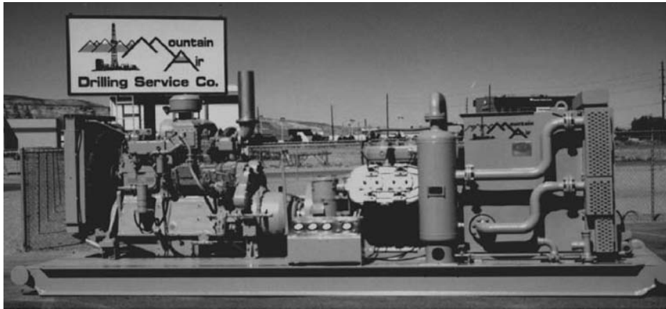
FIGURE 5-18. Skid-mounted, reciprocating piston primary compressor system unit (courtesy of Mountain Air Drilling Service).
