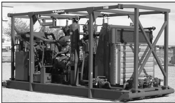
FIGURE 5-22. Skid-mounted, reciprocating piston low pressure booster compressor system unit (courtesy of Weatherford International).
