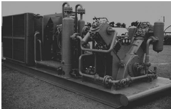
FIGURE 5-19. Skid-mounted, reciprocating piston booster compressor system unit (courtesy of Mountain Air Drilling Service).
