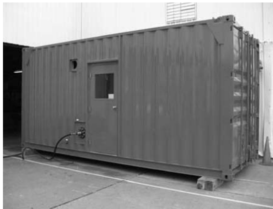
FIGURE 5-24. Typical membrane filter field unit for drilling operations (courtesy of Weatherford International).
