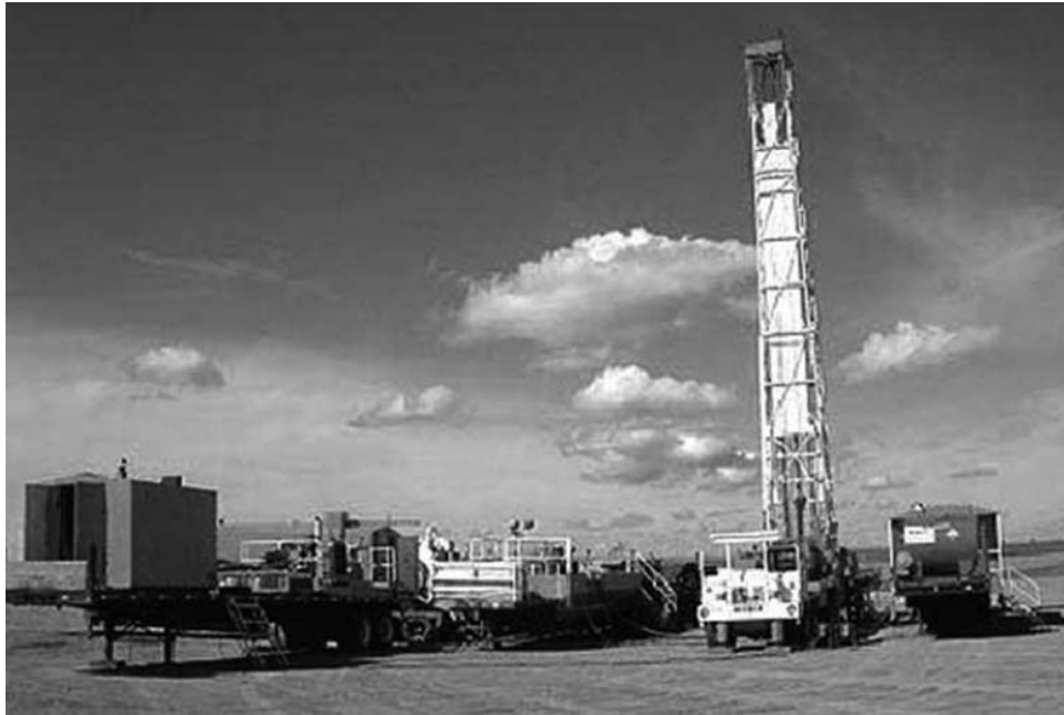
FIGURE 2-3. Typical self-propelled single drilling rig (courtesy of George E. Failing Company).
