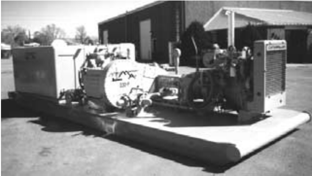
Figure 8-13: Liquid “mist” pump for air (or natural gas) drilling operations.
