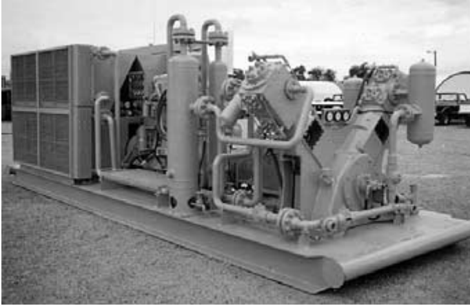
Figure 4-23: Skid mounted reciprocating piston booster compressor system unit (courtesy of Mountain Air Drilling Service).
