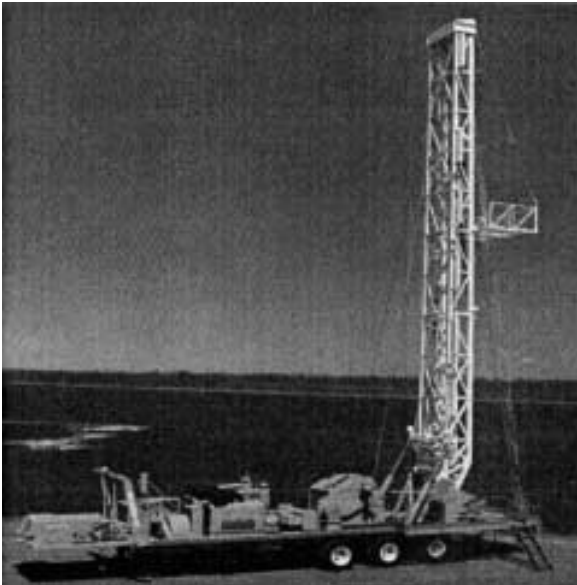
Figure 1-4: Typical trailer mounted drilling rig (courtesy of George E. Failing Company).
