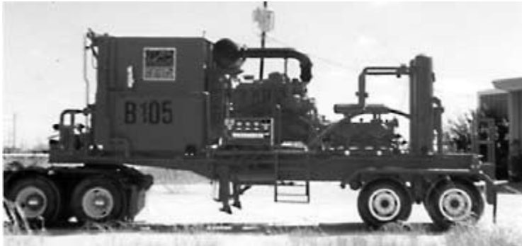
Figure 4-27: Skid mounted reciprocating piston booster compressor system unit (courtesy of Symbol Incorporated).
