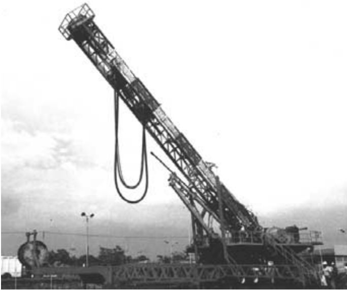
Figure 11-4: Trailer mounted slant capable deep drilling rig (courtesy of George E. Failing Supply Company, Limited).
