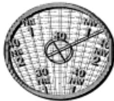
Figure 3-20: Typical single-shot exposure that reads north and 1.8° inclination from vertical (courtesy of Sperry-Sun Drilling Services, a Halliburton Company).
