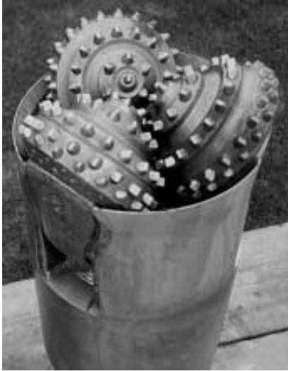
Figure 3-26: Skirted tri-cone roller cutter drill bit for dual pipe reverse circulation drilling operations (courtesy of Lang Exploratory Drilling).
