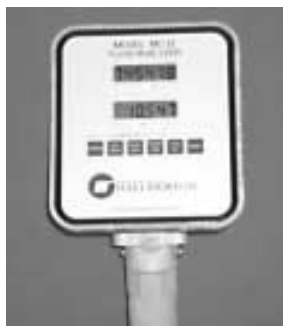
Figure 2-6: Digital display for the turbine flow meter (courtesy of Halliburton Energy Services, Incorporated).
