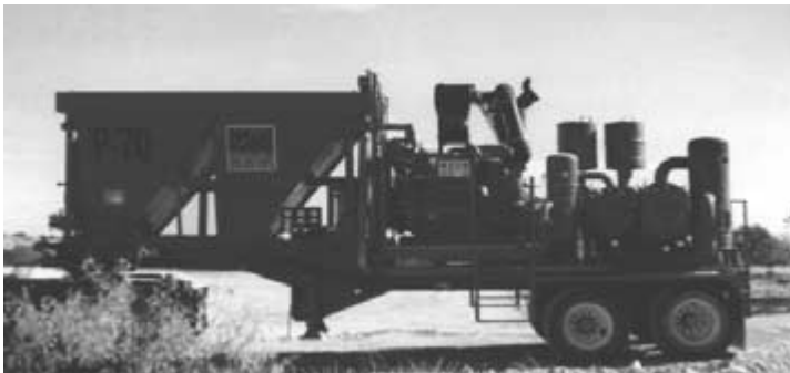
Figure 4-26: Semi-trailer mounted reciprocating piston primary compressor system unit (courtesy of Symbol Incorporated)
