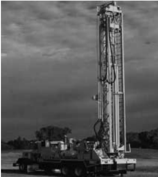
Figure 1-3: Typical self-propelled single drilling rig (courtesy of George E. Failing Company).
