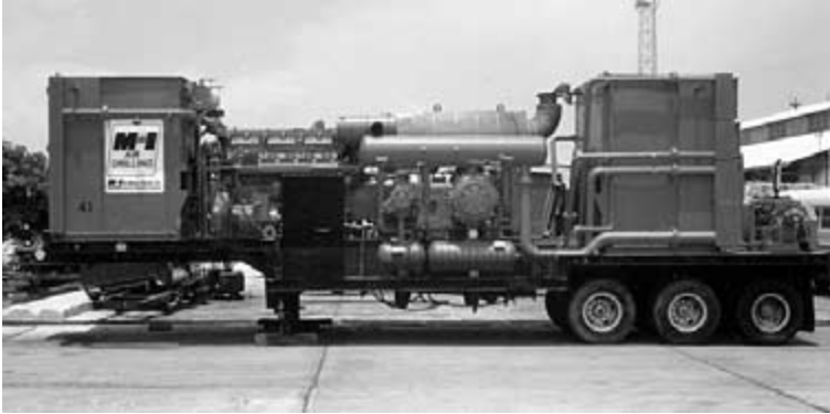
Figure 4-25: Semi-trailer mounted four-stage reciprocating piston compressor system unit (courtesy of MI Air Drilling).
