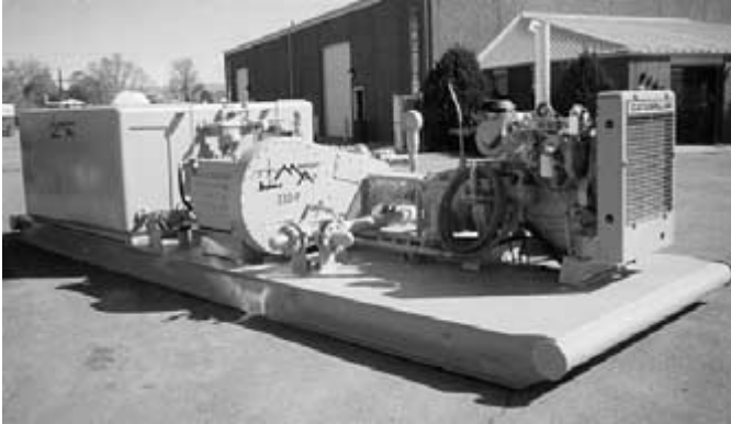
Figure 2-2: Water injection pump (courtesy of Mountain Air Drilling Services).
