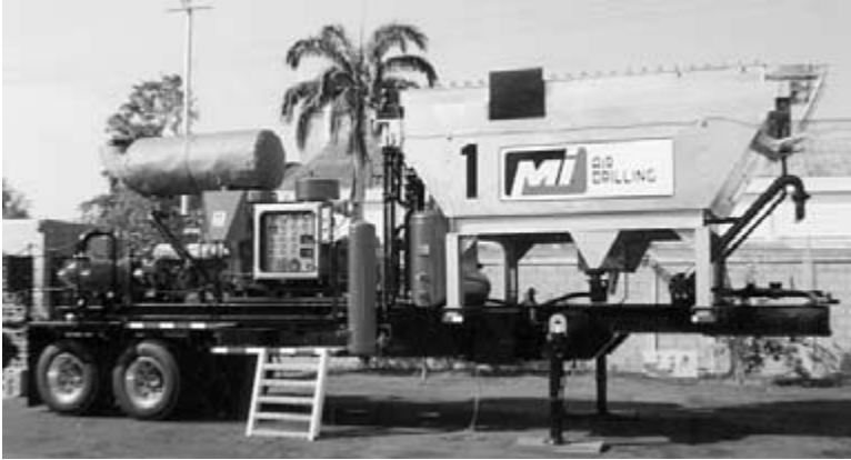
Figure 4-24: Semi-trailer mounted rotary primary and reciprocating booster compressor system unit (courtesy of MI Air Drilling).
