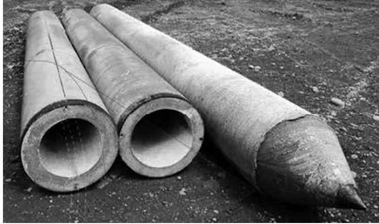
Figure 16.6 Example of hollow precast reinforced concrete energy piles prior to their installation on site, piping equipment and filling with appropriate material. Image courtesy: SACAC.
