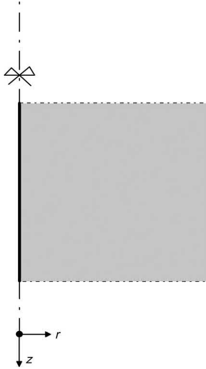
Figure 9.9 Schematic of the infinite line source model.
