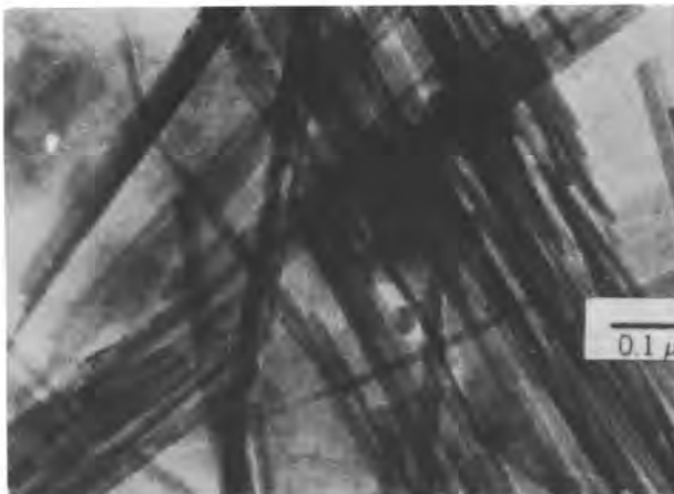
Fig. 2.18—Transmission electron micrographs of attapulgite (left) and sepiolite (right). 4
