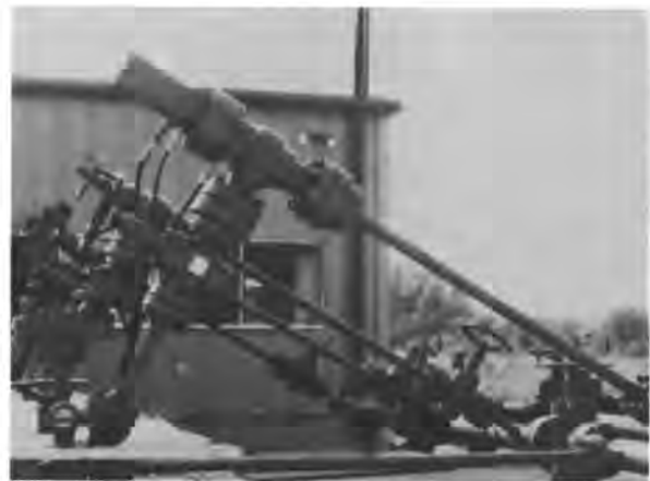
Fig. 1.52 – Example choke manifold showing 15,000-psi hand-adjustable choke and 15,000-psi remote adjustable choke.
