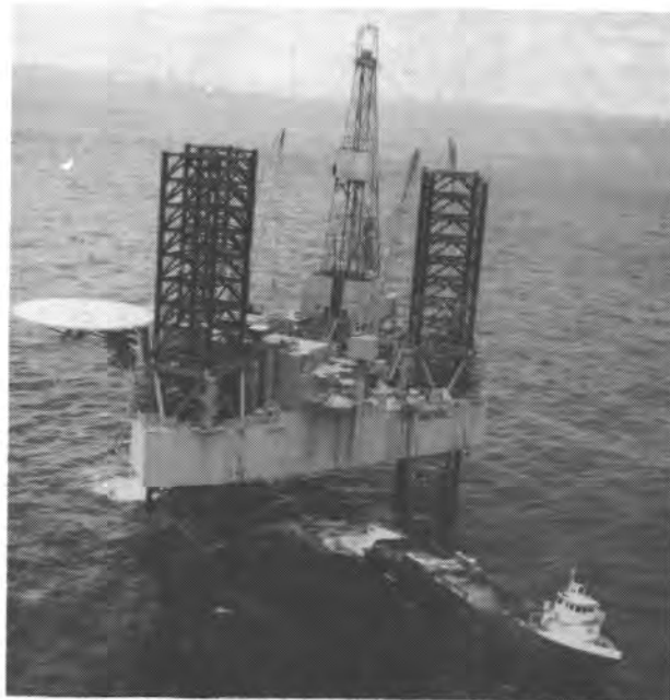
Fig. 1.8—Jackup rig Mr. Mel on location in the Eugene Island area, offshore Louisiana.
