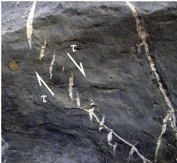
Figure 3.18 Field example of shear failures in sigmoidal veins (Bons et al., 2012).
