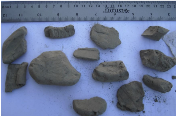
Figure 10.10 Large size cuttings from a gumbo shale at a depth of \sim 7300 ft TVD KB for drilling with a PDC bit in the Gulf of Mexico.
