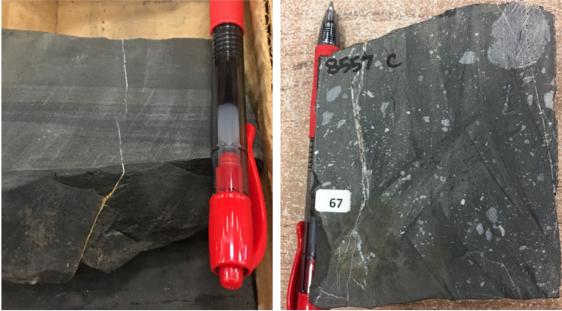
Figure 4.14 Core pictures of the Wolfcamp C showing partially filled natural fractures perpendicular to the bedding planes.
