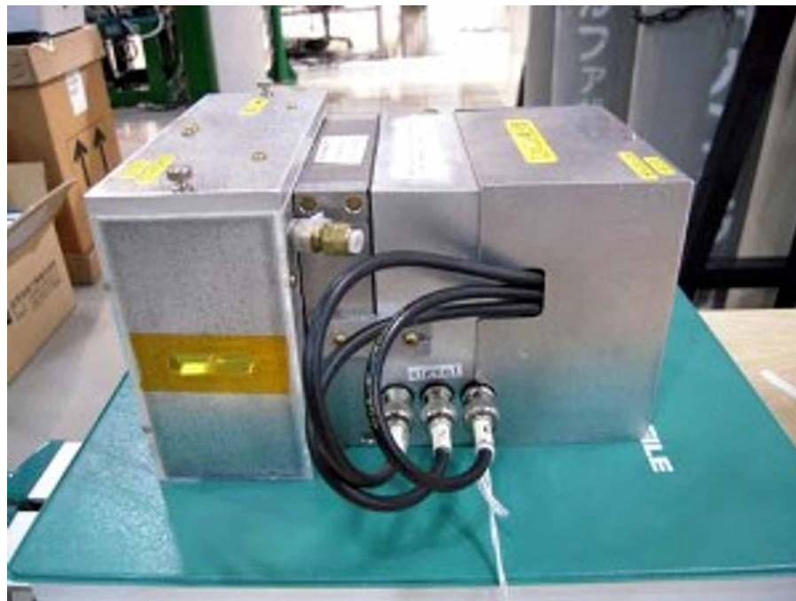
Figure 7. A fluorescence Lytle detector ( http://www.saga-ls.jp )
