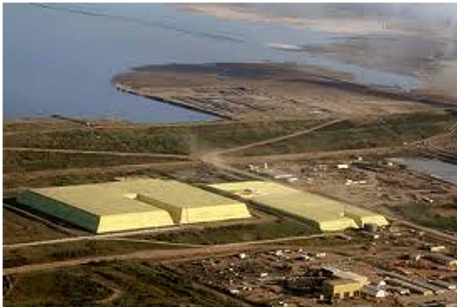
Figure 1. Sulfur removal from Athabasca bitumen is stored as elemental sulfur in exposed enormous yellow mounds
