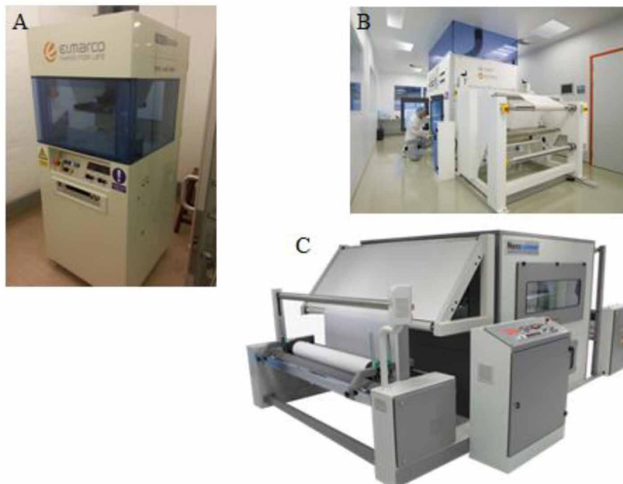
Figure 11. (A) Elmarco laboratory-scale electrospinning apparatus; (B) industrial-scale electrospinning system, Nanospider produced by Elmarco ( http://www.elmarco.com/nanofiber-equipment/electrospinning-machines-ns1ws500u/ ); (C) industrial-scale electrospinning system, Nanospinner416 produced by Inovenso Ltd. ( http://www.inovenso.com/portfolio-view/nanospinner416/ )
