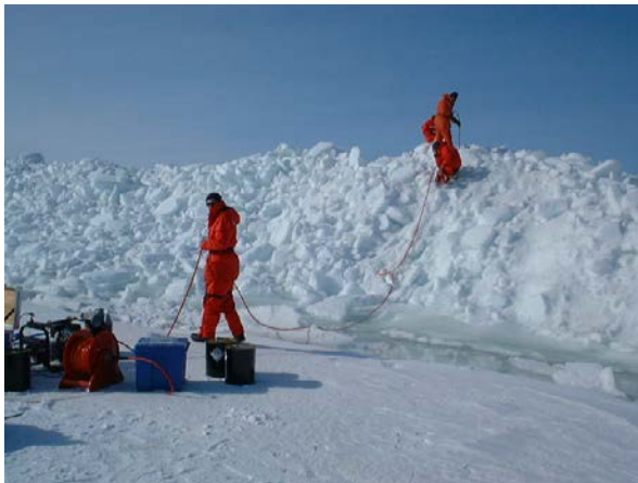
Figure 2.5 Thermal drill in use on small stamukha (Photo by KRCA)
