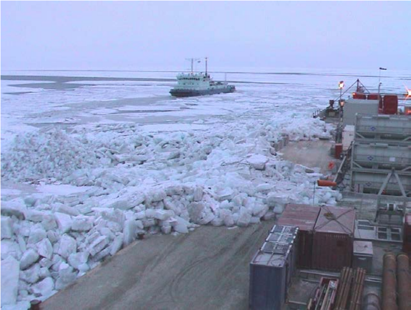
Figure 4.23 Ice over-ride incident in the Caspian Sea (from McKenna et al.[69])
