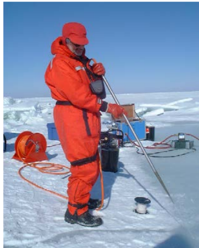
Figure 2.4 Thermal drill probe (Photo by KRCA)
