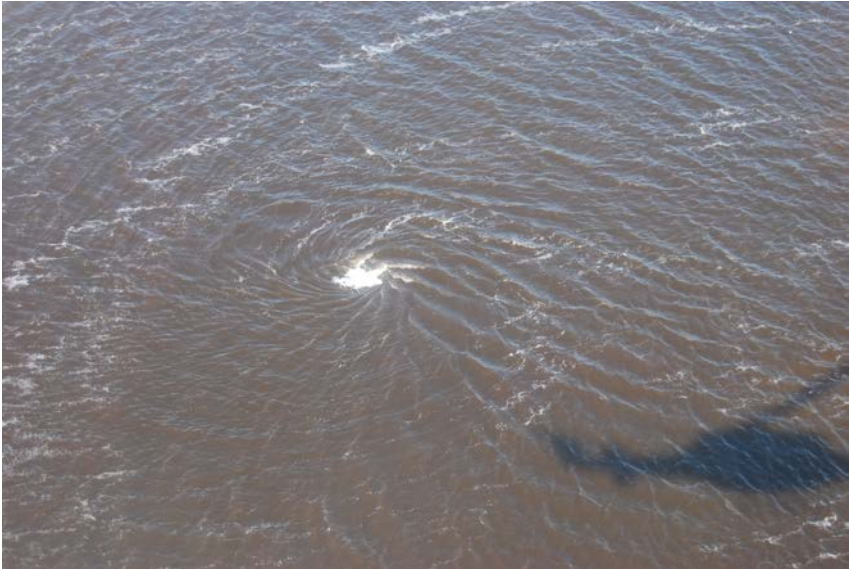
Figure 7.6 Strudel scour (photo by courtesy of Craig Leidersdorf, Coastal Frontiers)
