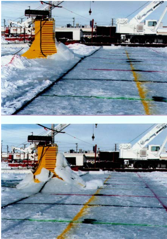
Figure 4.17 Ice breaking and ride-up in tests in the Esso basin in 1989 [63] (with permission of Imperial Oil, Calgary)
