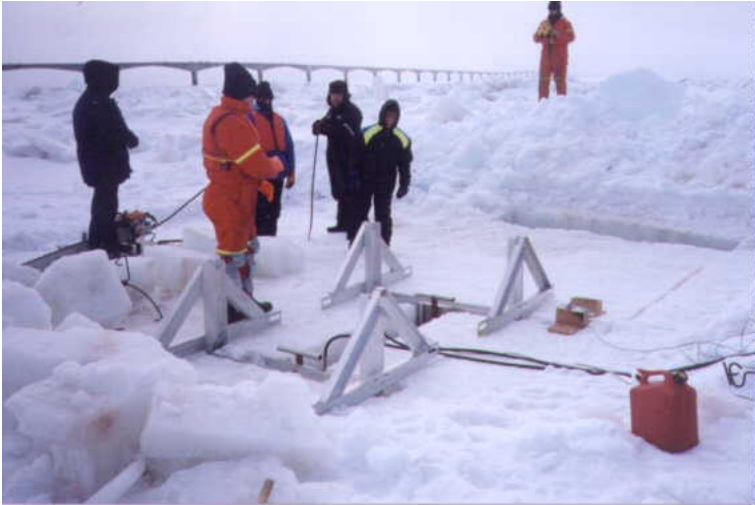
Figure 3.9 Direct shear test (Confederation Bridge in background) (photo by KRCA)
