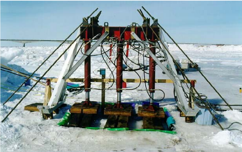
Figure 3.12 Punch shear test apparatus as used in Canada in 1998 (photo by KRCA)
