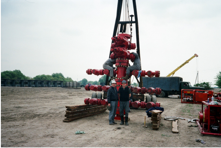
Fig. 6.24 Capping stack with flange on bottom.
