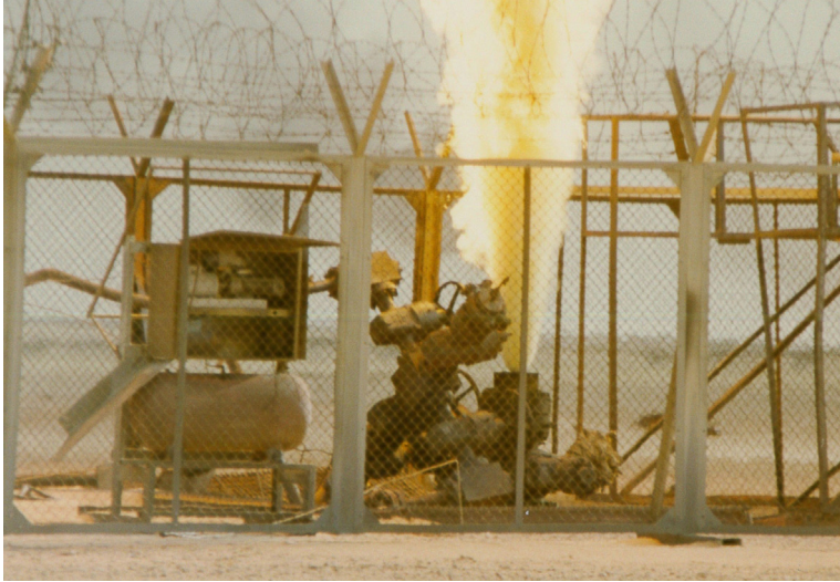
Fig. 11.5 Tree blown off with complete combustion.
