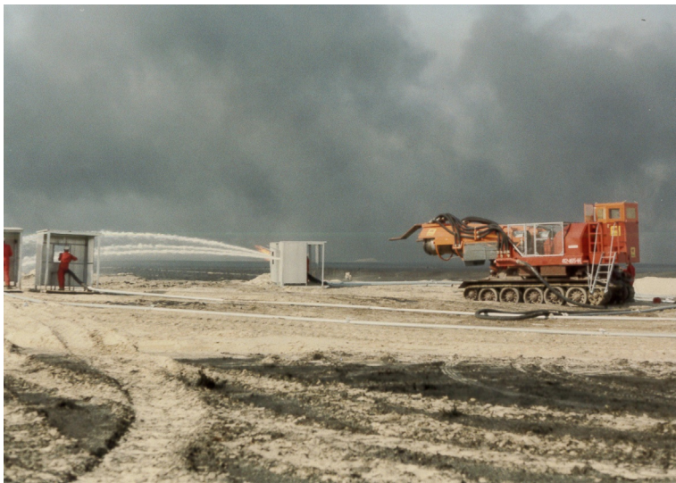
Fig. 4 Hungarian “Big Wind” for blowing out the fire with jet engines.
