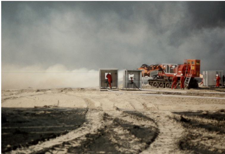
Fig. 11.19 Blowing out a fire with jet engines.
