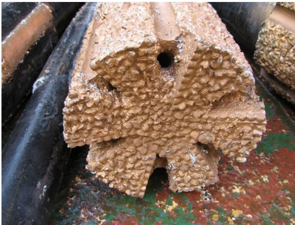
Fig. 7.2 Typical intercept mill.
