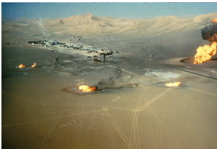
Fig. 8.15 Well cratered at a water well 127 m away in Algeria.
