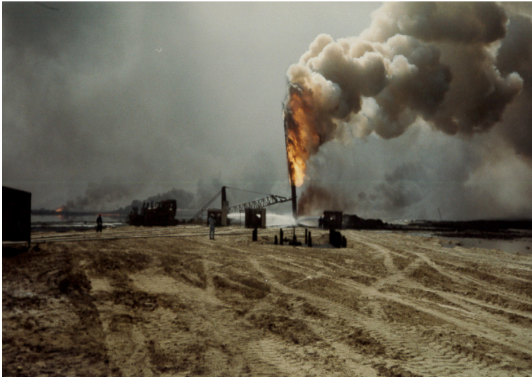
Fig. 11.17 Extinguishing a fire with water.
