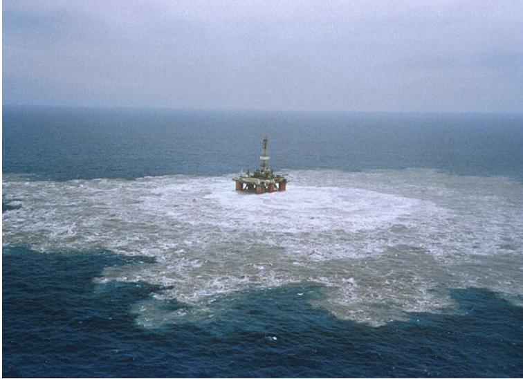
Fig. 8.2 Underground blowout with a semisubmersible.
