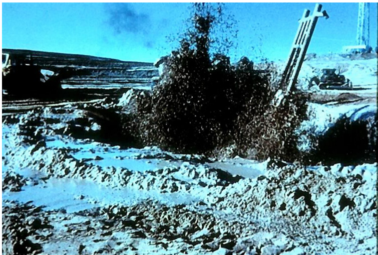
Fig. 8.14 Apache Key well cratered at the wellhead.
