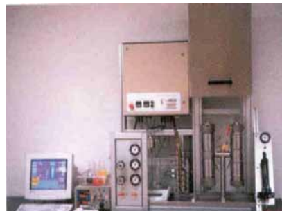
Fig. 3.9—Coreflood tester showing schematic and a photo.
