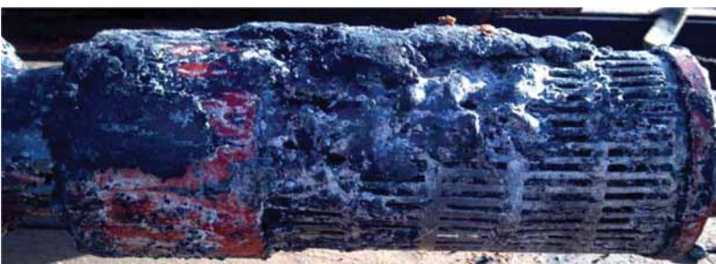
Fig. 2.26—Asphaltene and calcite scale on ESP screen (anonymous producer).
