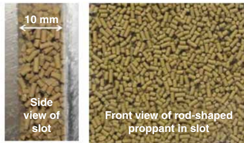
Fig. 4.73—Views of random alignment of rods after settling in a slot (McDaniel et al. 2010).
