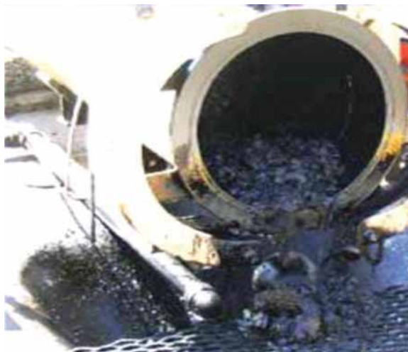
Fig. 2.25—Mixed deposit in pipeline (Bell et al. 2008). Photograph courtesy of Rick Armstrong.
