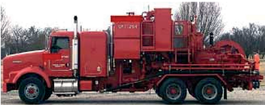
Fig. 1.43—Pumper for matrix acid and cement placement (Halliburton 2006).
