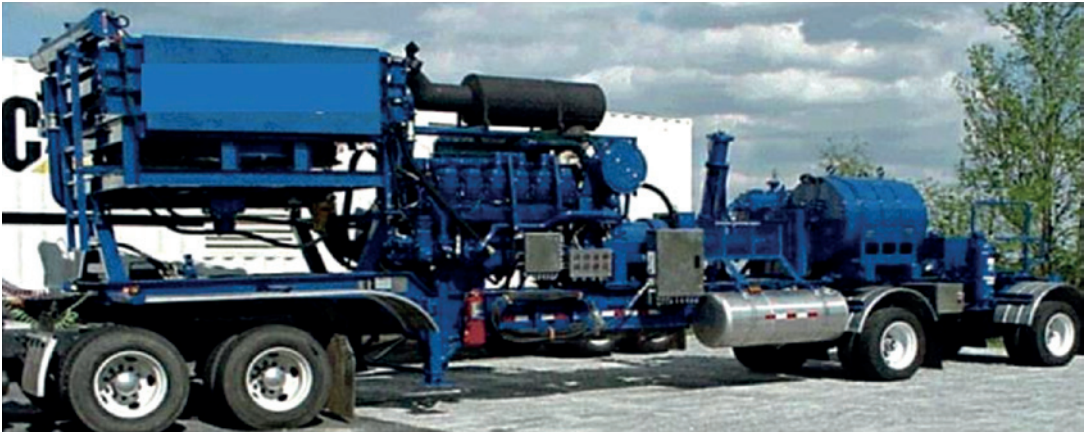
Fig. 1.44—Portable high pressure frac pump (Schlumberger).
