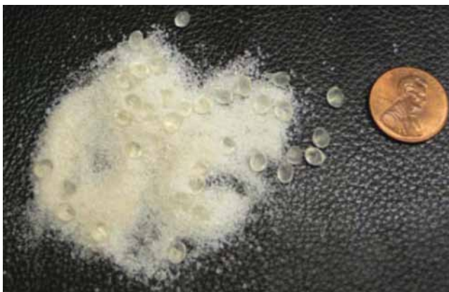
Fig. 3.79—Biodegradable particle diverting agent (Denney 2011).
