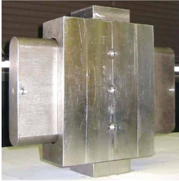
Fig. 3.101—Modified API cell for acid frac conductivity tests (Zou 2006).
