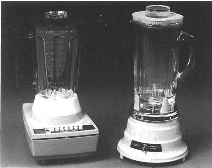
FIGURE 3.3 High-speed blenders. Narrow clearance between blades and baffles results in high shear rates. Courtesy of Fann Instrument Company.
