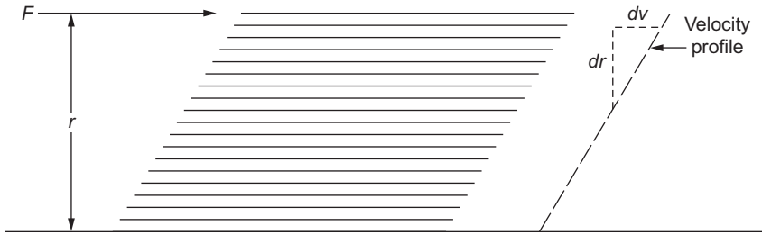
FIGURE 6.2 Schematic illustration of laminar flow of a Newtonian liquid.
