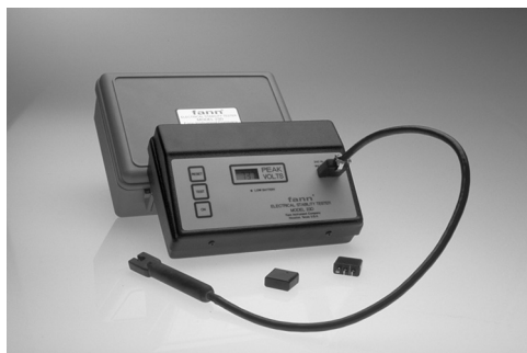
FIGURE 3.19 Electrical stability meter for NADF. Courtesy of OFI Testing Equipment.
