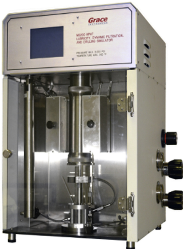
FIGURE 3.15 M2200 HPHT lubricity, dynamic filtration, and drilling simulator. Courtesy of Grace Instruments, Inc.
