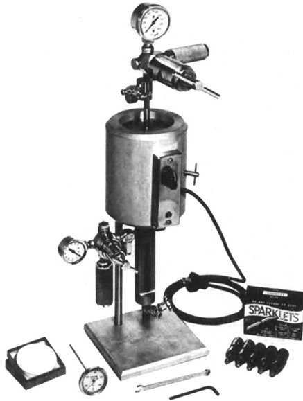
FIGURE 3.12 HPHT filter tester with pressure receiver—175 mL volume. Courtesy of Fann Instrument Company.
