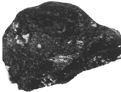
FIGURE 9.36 Destabilization of shale specimen by penetration of water along microfractures. Apparently competent specimen brought up in junk basket in air-drilled hole.
