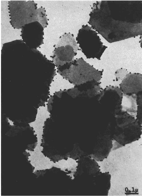
FIGURE 4.17 Electron micrograph of a mixture of kaolinite and a gold sol. From van Olphen, H., 1977. An Introduction to Clay Colloid Chemistry , second ed. John Wiley & Sons, New York, photographed by H.P. Studer. Courtesy of John Wiley & Sons.
