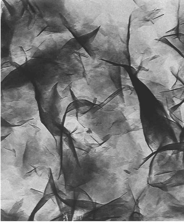
FIGURE 4.7 Electron micrograph of montmorillonite. Magnification \times 87,500 . Courtesy of J.L. McAtee, Baylor University.
