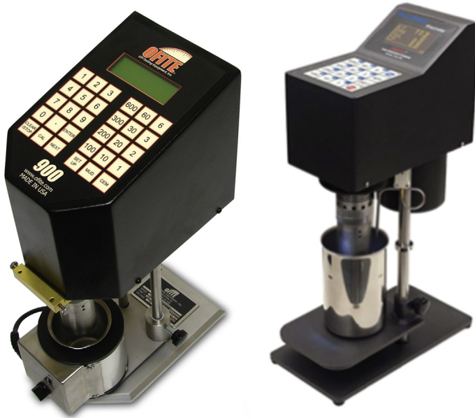
FIGURE 3.10 Continuous speed viscometers. (A) OFI Testing Equipment Model 900 viscometer and (B) Fann Instrument Company RheoVADR rheometer.
