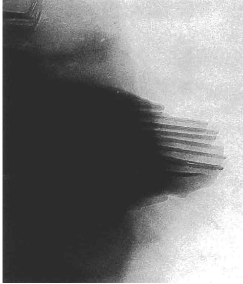
FIGURE 4.8 Edge view of a flake of sodium montmorillonite. The dark parallel lines, which are 10 \text{ \AA} \pm thick, are the unit layers. Electron micrograph by Barclay, L.M. and Thompson, D.W., 1969. Electron microscopy of montmorillonite. Nature 222, 263. Courtesy of Nature.
