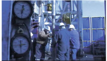
(p) Replacing the lift bail with the top sub
