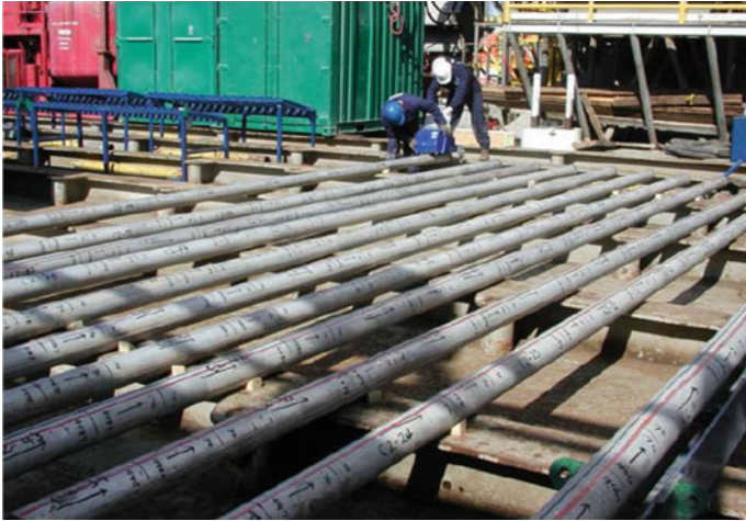
Fig. 14.14 Gamma-ray logging of the core at the surface, which is done before cutting the inner tube joints into one-meter sections (published courtesy of Baker Hughes GE)
