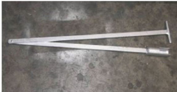
Fig. 14.1 Drop-ball pick-up tool to extract the ball stuck inside the inner tube (published courtesy of Baker Hughes GE)
