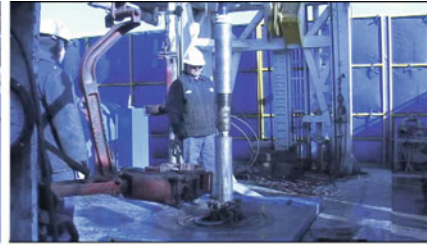
(j) Disconnect the top joint of the outer tube
