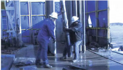
(c) Hold the outer tube near the rotary table, disconnect the protector bottom sub
