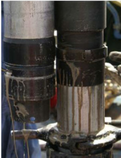
Fig. 14.11 a After cutting the core at the bottom of the inner tube joint, it is secured by placing the cap and cushion on the bottom (of the upper half of NRITS), and the splitter is detached or removed from the inner tube joint, b the inner tubes to be cut, the left is a cut and secured inner tube, which is going to be loaded and attached to the LDF for transportation to the pipe-decks/ground (published courtesy of Baker Hughes GE)
