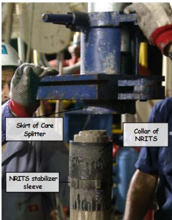
Fig. 14.10 The inner tube joint (with NRITS between every two joints) has been cut by the splitter (published courtesy of Baker Hughes GE)
