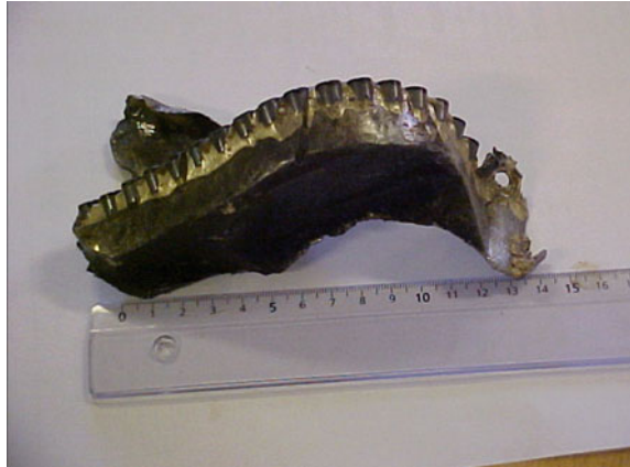
Fig. 5.4 A bit blade as the junk riding on top of the core sample (photo published courtesy of Baker Hughes GE)
