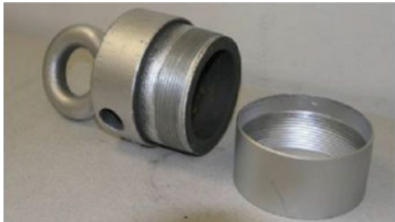
Fig. 14.2 The inner tube lift bail , which is used for lifting the inner tube out of the hole (published courtesy of Baker Hughes GE)
