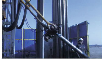
(b) Using tuggar line and then elevator to carry the outer tube to the floor
