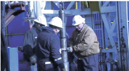
(o) Using clamps to take inner tube on the outer tube and letting the lift bail to be released
