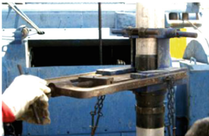
Fig. 14.8 Mechanical core splitter/guillotine, which is mechanically turned between the inner tube joints in order to cut the disposable inner liner/core (published courtesy of Baker Hughes GE)
