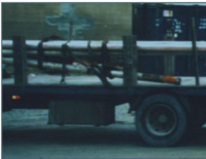
Fig. 14.17 Inappropriate transportation of the inner tubes to the central laboratory. In this example, it is seen that even cutting of the long inner tube into sections has not been done (Hettema et al. 2002)
