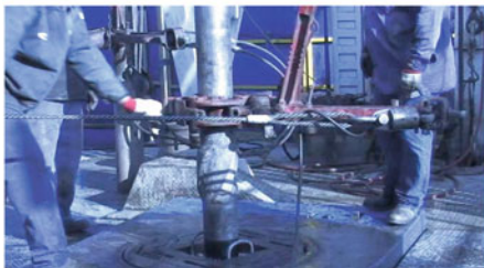
(g) Use rig tongs to apply torque
