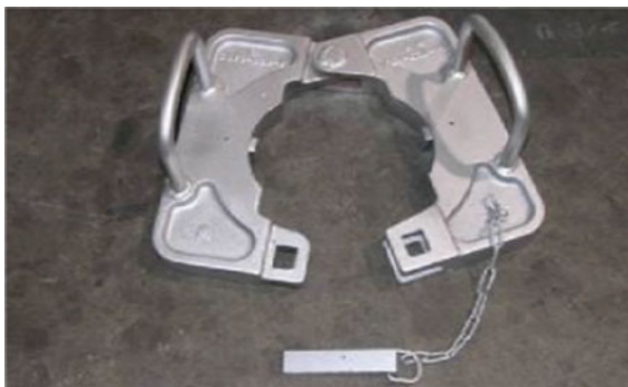
Fig. 14.3 The bit breaker, used to remove the core bit (published courtesy of Baker Hughes GE)
