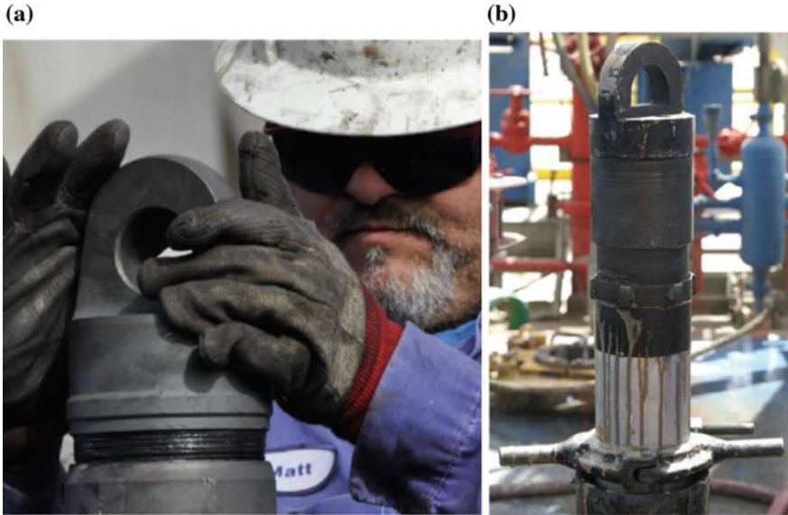
Fig. 14.6 In conventional coring, the lift bail/sub is connected to the top of the inner tube and is raised using the tugger line to pull the next inner tube out of the outer tube. Now, the same cutting and lay-down process can be repeated for this inner tube joint (published courtesy of Baker Hughes GE)
