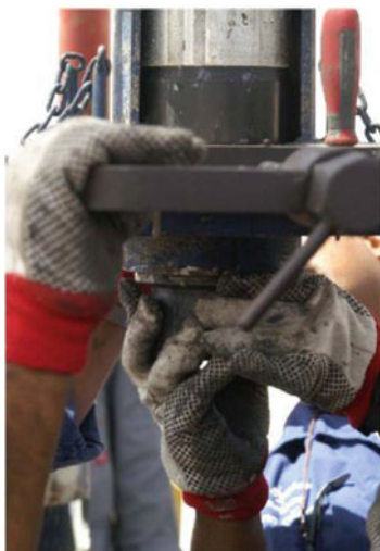
Fig. 14.11 a After cutting the core at the bottom of the inner tube joint, it is secured by placing the cap and cushion on the bottom (of the upper half of NRITS), and the splitter is detached or removed from the inner tube joint, b the inner tubes to be cut, the left is a cut and secured inner tube, which is going to be loaded and attached to the LDF for transportation to the pipe-decks/ground (published courtesy of Baker Hughes GE)
