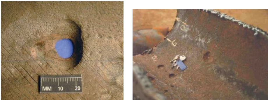
Figure 11.1 Typical features of MIC type damage characteristic of localised morphologies. (see colour plate section).
