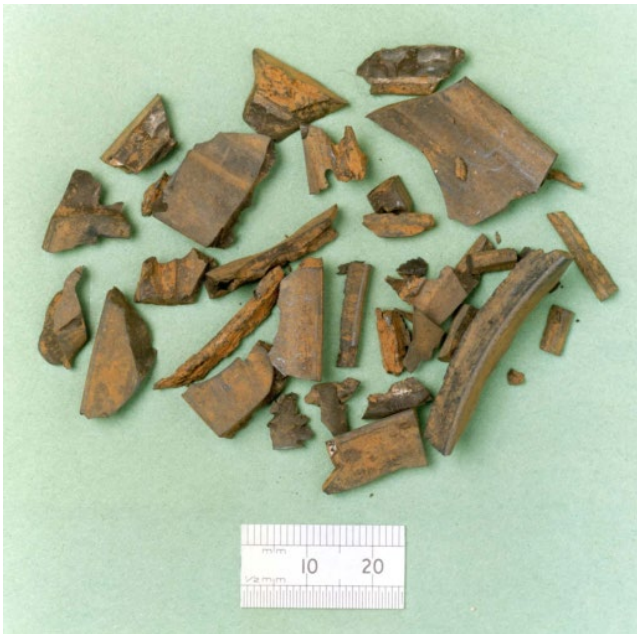
Figure 15.1 An example of heat ageing of a rubber seal. (see colour plate section).
