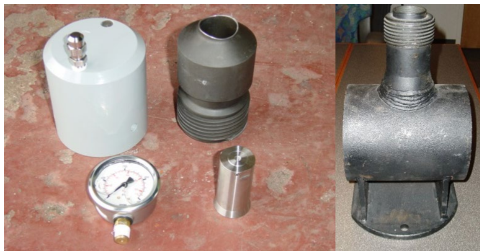
Figure 10.2 Access fitting: kit and example installation. (see colour plate section).
