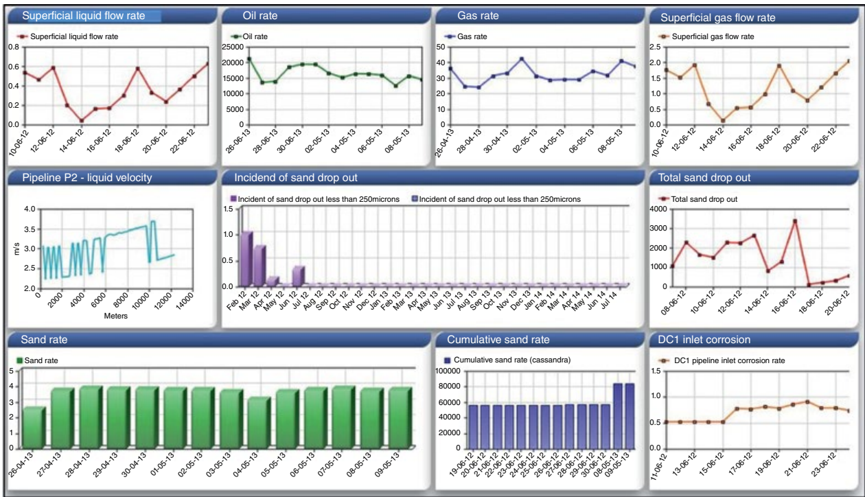
Figure 10.4 An example of a corrosion management dashboard.
