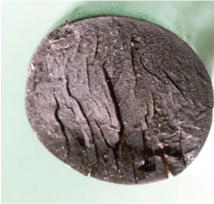
Figure 15.3 Examples of decompression damage to rubber.
