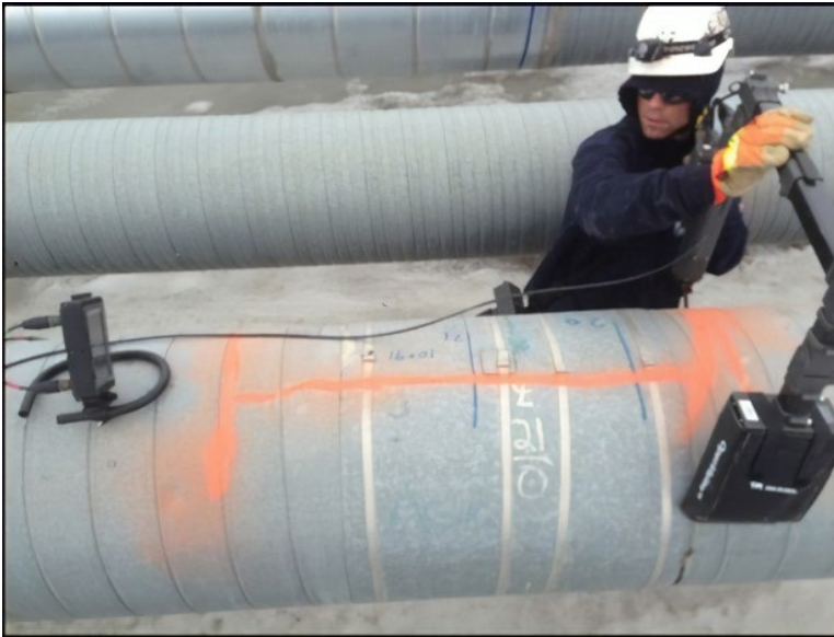
Figure 10.5 A one-person-operated, portable RT unit in use. (see colour plate section).
