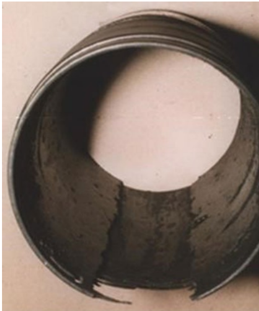
Figure 17.2 An example of bottom of line groove corrosion.
