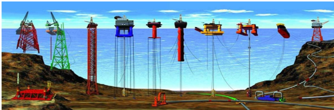
Figure 6.2 Various types of offshore structures and their typical locations.
