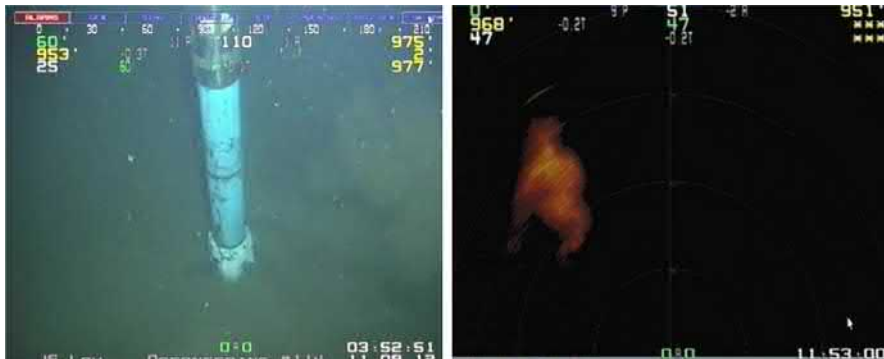
FIG. 13.1 Deepwater 12¼" pilot hole to evaluate presence of shallow hazards. Source: Kingdom Drilling training 2014.
