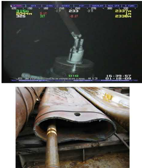
FIG. 13.18 Deepwater Conductor jetting failures. Source: Kingdom Drilling training 2014.
