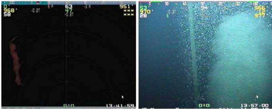
FIG. 13.2 Deepwater 12 ¼" pilot hole to determine and evaluate the presence of shallow hazards. Source: Kingdom Drilling training 2014.
