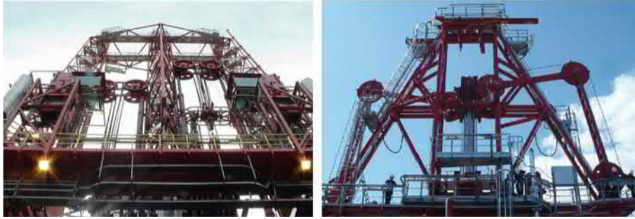
FIG. 5.26 Hydraulic ram rig compensation (left image) and Crown-mounted compensation system (right image). Source: Kingdom Drilling training 2009.
