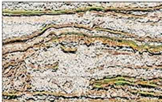
FIG. 12.4 Gulf of Mexico, 3D seismic, channelized sand “shallow flow” hazard presence. Source: Kingdom Drilling training 2002.
