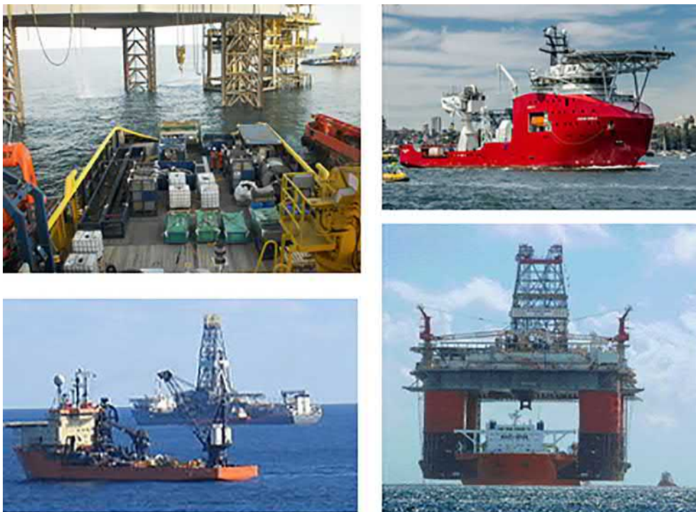
FIG. 5.47 Supply (top left), intervention (top right), stand-by/emergency response (bottom left), rig move (bottom right) vessels. Source: Photographs are from unknown providers as licensed under CC BY-SA .
