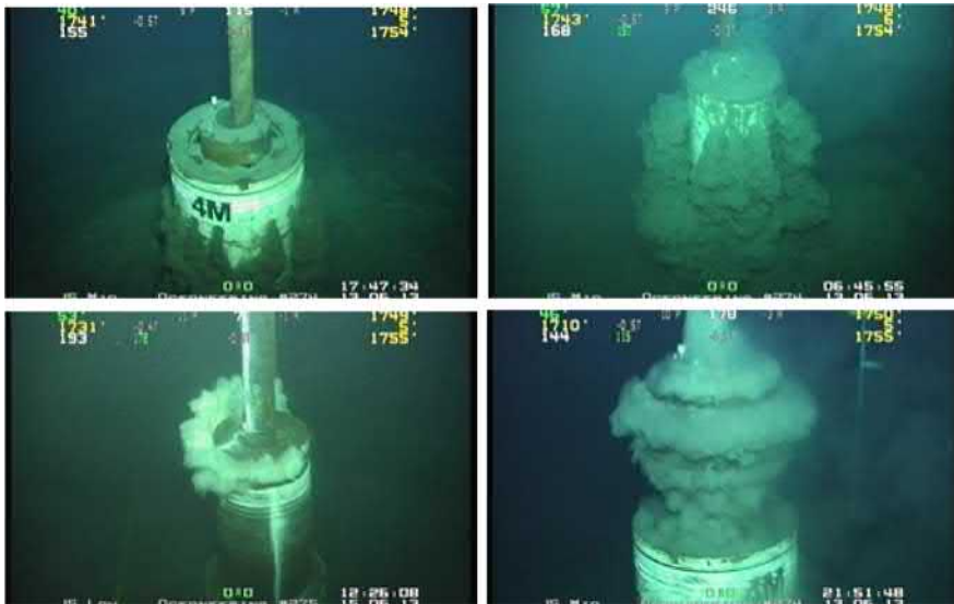
FIG. 13.16 Drilling ahead and releasing tool and pulling BHA at end of surface wellbore section drilling. Source: Kingdom Drilling training 2014.
