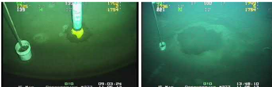
FIG. 13.13 ROV snapshot of a penetration test, in 1752m water depth being and end 4h, 45min later. Source: Kingdom Drilling training 2014.
