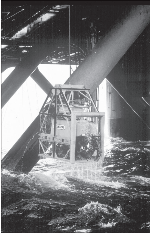
Fig. 13–11. ROV in its cage being launched. (Courtesy Oceaneering.)
