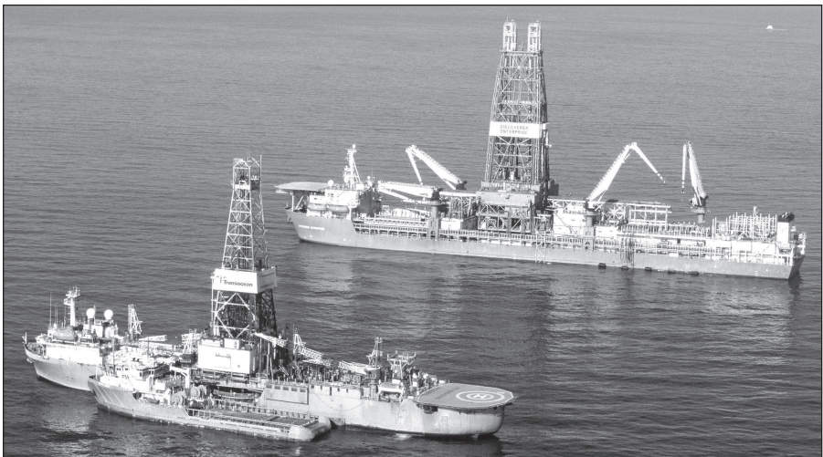
Fig. 5–7. The larger drillship, Discoverer Enterprise has a dual activity facility. The smaller, earlier vintage drillship, is the Discoverer 534 , alongside a supply boat.
