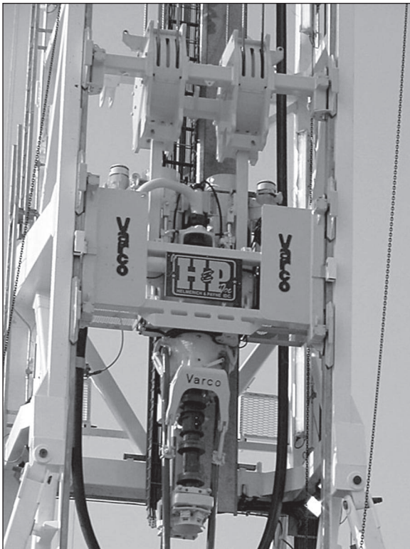
Fig. 5–2. A top drive on a track in the derrick. It moves up and down in the derrick and turns the drill pipe and drill bit.
