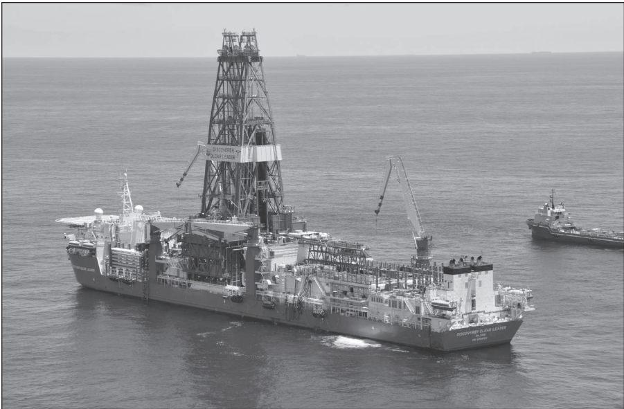
Fig. 6–4. The drillship Discoverer Clear Leader , showing the dual activity mast
