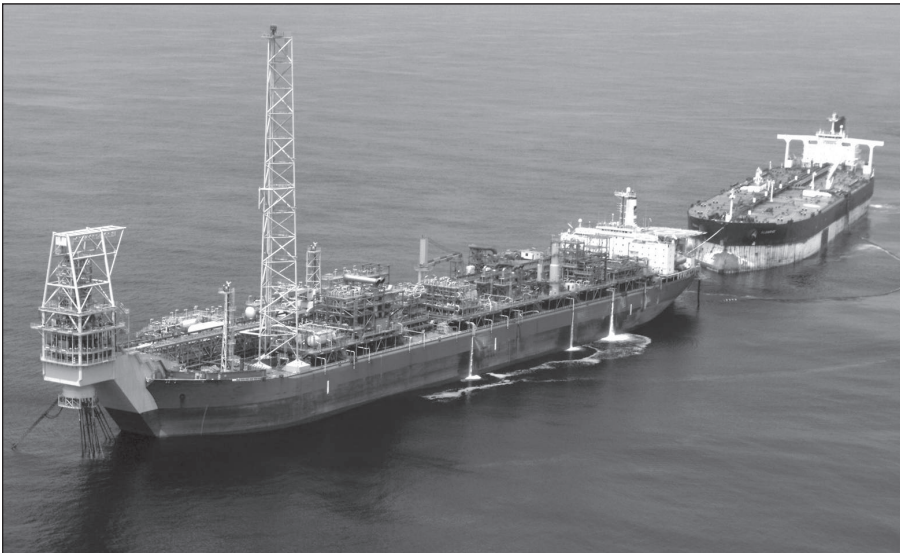
Fig. 9-16. Weathervane, external turret, and swivel system. (Courtesy SBM Offshore.)
