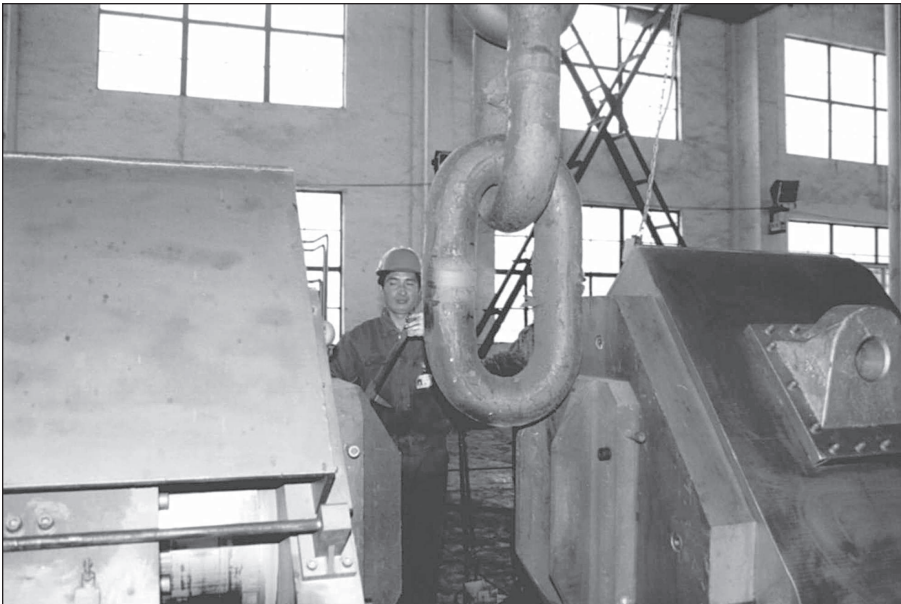
Fig. 9–26. A 500-pound chain link for a mooring chain. (Courtesy Offspring International.)
