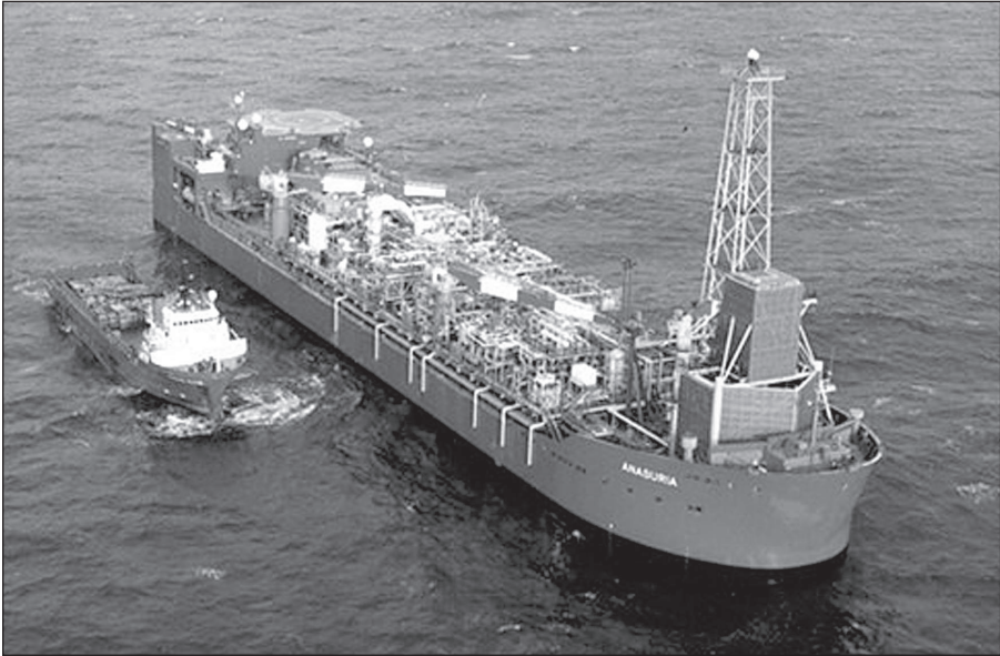
Fig. 9–13. The FPSO Anasuria in the North Sea. (Courtesy Shell International.)
