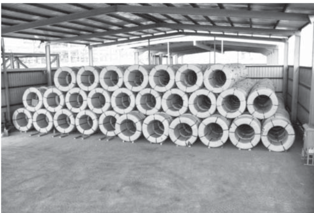
Fig. 8.19 Storage of prestressing strands.
