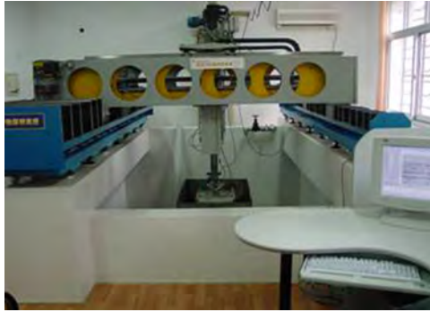
Figure 2.7 3D high-precision positioning and observation instrument.
