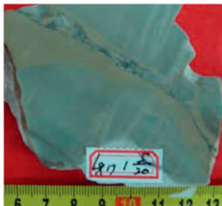
Figure 1.53 Fillings in solution fractures. Grayish-yellow calcareous-argillaceous filling materials in earlier stages and calcite in later stages.
