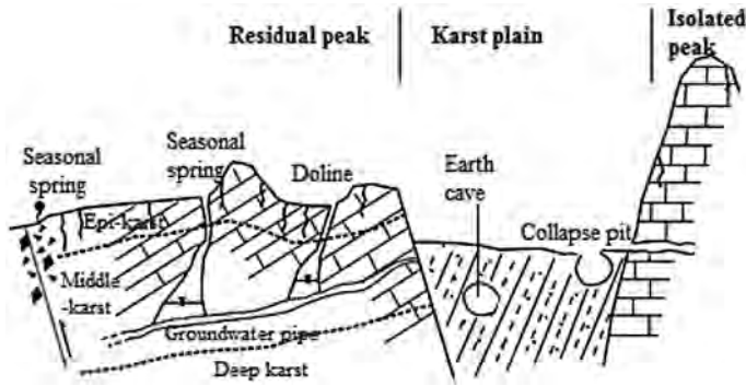
Figure 1.5 Morphology of karst in regions with different topography and geomorphology (Riyuan et al., 2011).
