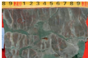
Figure 1.51 Fractures and vugs filled with light-green calcareous-argillaceous siltstone in Well S79.
