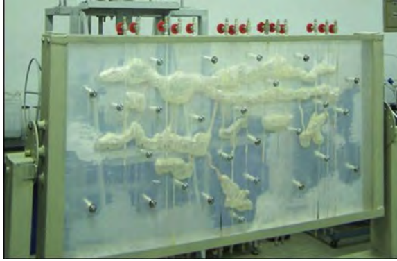
Figure 5.21 Physical experimental modeling of fracture-vug reservoir.
