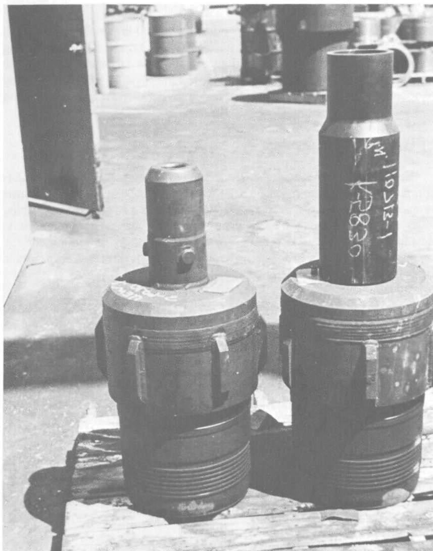
FIG. 6-2 20-in. mud-line corrosion cap and running tool. (Courtesy Vetco)
