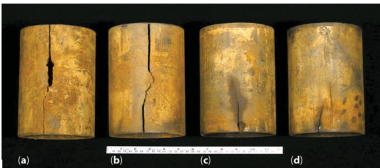
Figure 6.15 Pipe failure due to twist-off and/or fatigue.
