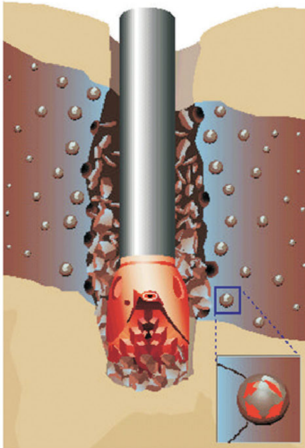
Figure 9.7 Drilling through induced over-pressured shale.
