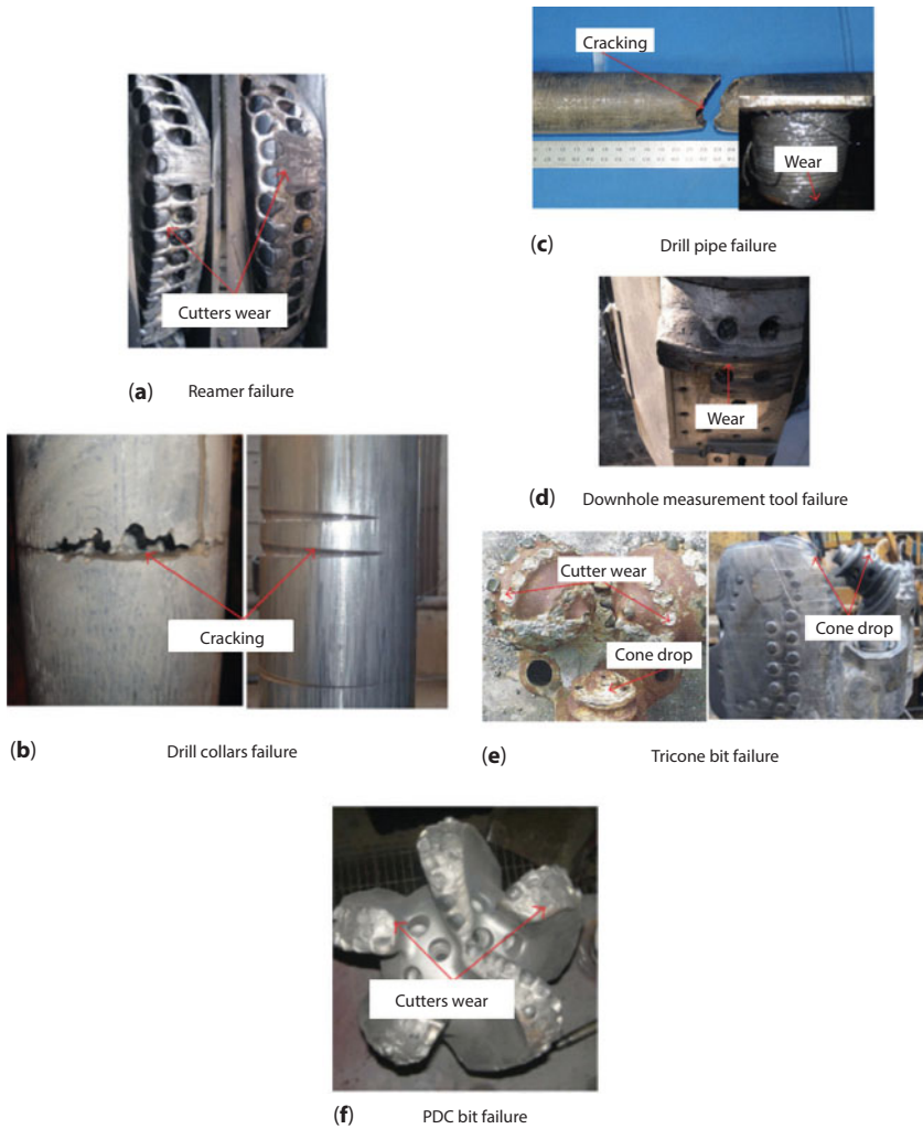
Picture 6.2 Damages caused by V&S in different drillstring components (Dong et al. , 2016).
