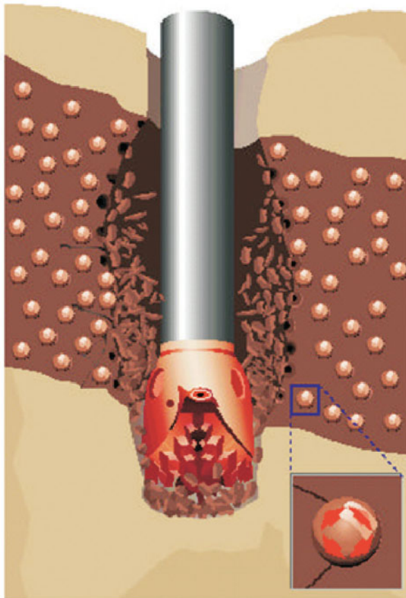
Figure 9.6 Drilling through a naturally overpressured shale.
