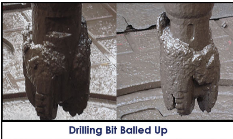
Figure 2.24 Drilling bit balled up.
