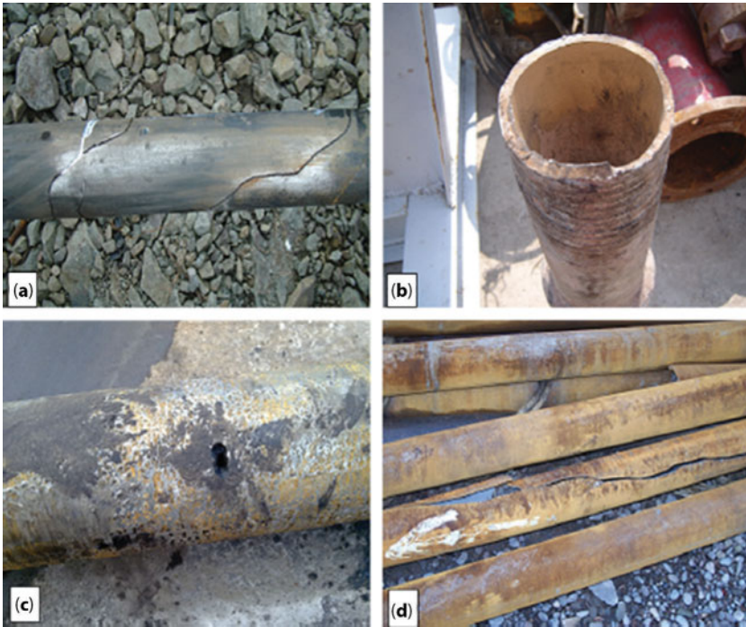
Picture 4.1 Photos of typical drillstring failure: (a) fatigue fracture of drillstring caused by gas drilling; (b) fracture surface of drillstring; (c) the washout of drillstring due to corrosion; (d) fracture of drillstring due to hydrogen embrittlement. (From Wang et al. , 2011).
