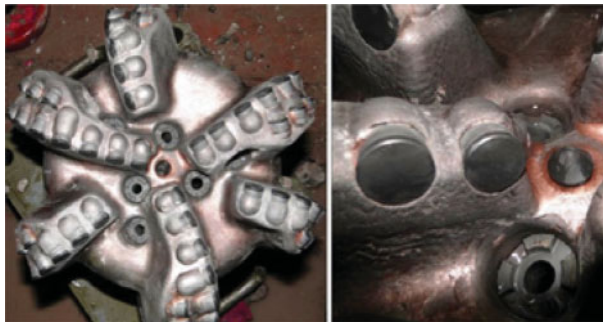
Figure 2.23 Stinger bit crush and shear the cuttings.
