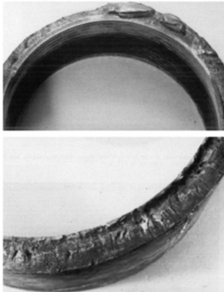
Figure 6.19 Post-separation damage to fracture surfaces of a BHA connection. (Macdonald 2007).
