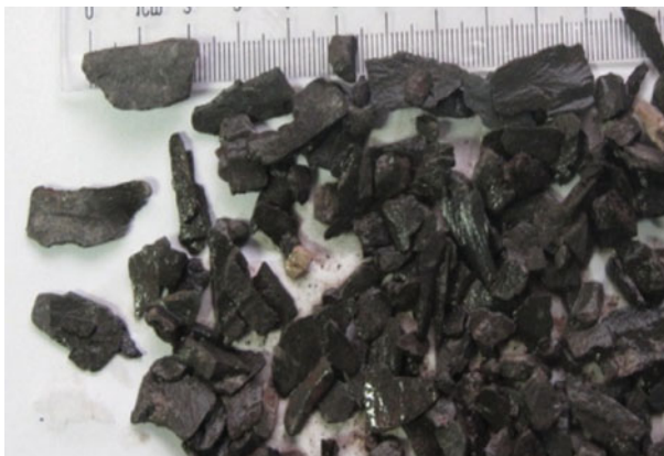
Picture 9.2 The shale cavings of the Nahr Umr Shale of N006H Well.
