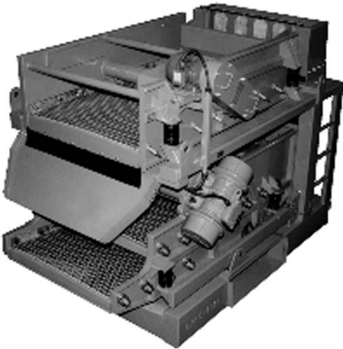
Figure 7.19. Integral cascade unit with multiple vibratory motions.
