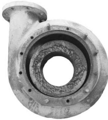
Figure 18.14. Results of abrasive fluid cavitation.
