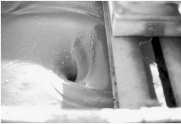
Figure 10.10. Vortex formation in fluid.
