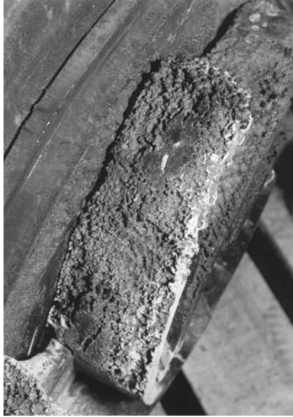
Figure 18.12. Results of clear fluid cavitation.
