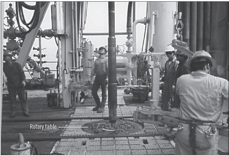
Fig. 5–21. Drill floor and rotary table with the drillstring hanging in slips
