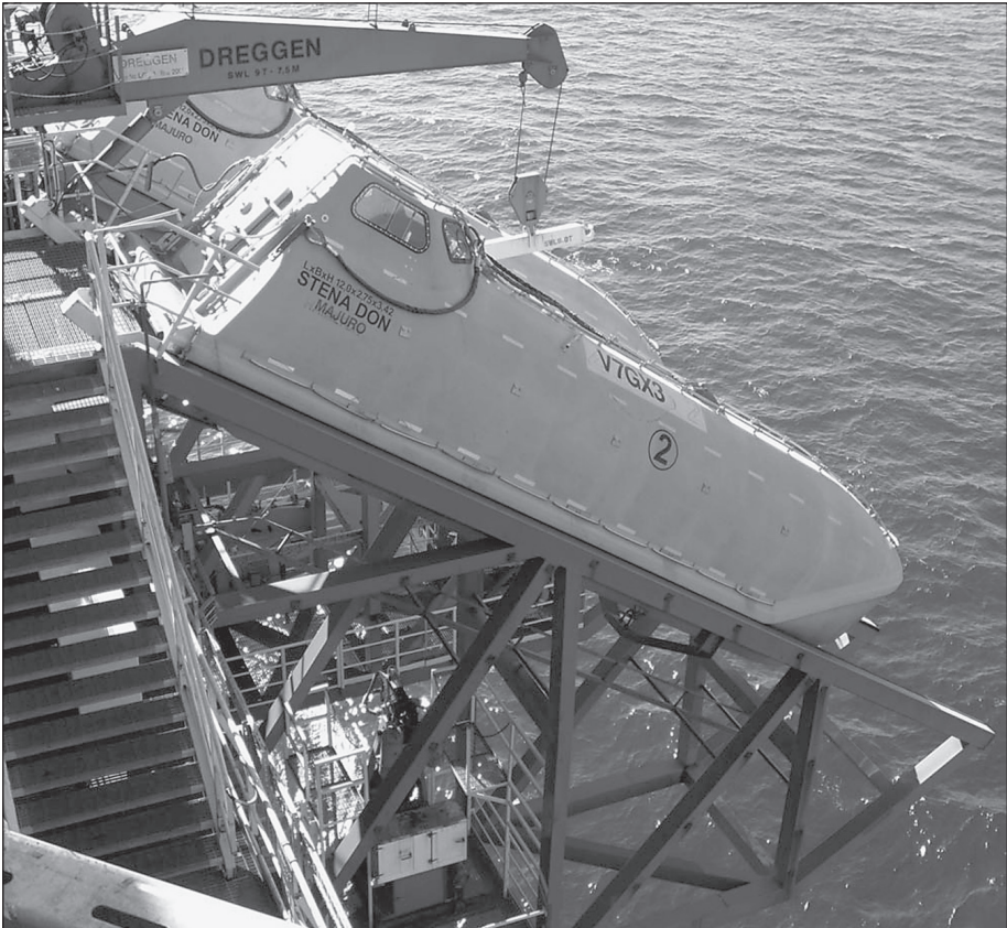
Fig. 14–1. Lifeboat on a semisubmersible rig
