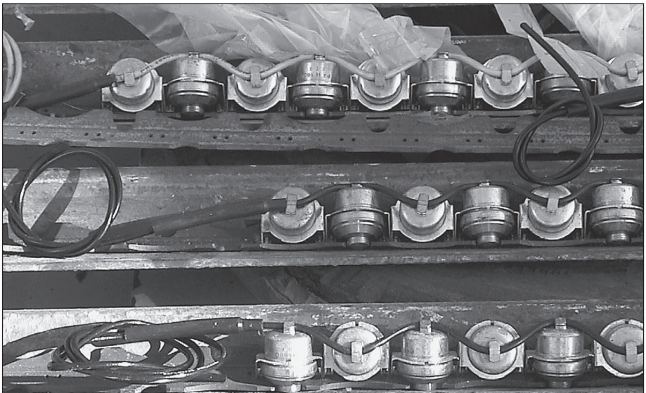
Fig. 9–3. Perforation charges being loaded
