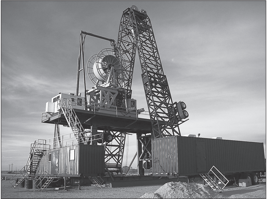
Fig. 5–5. Rotating coiled tubing rig near Odessa, Texas
