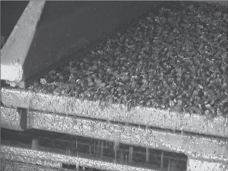
Fig. 10–1. Drilled cuttings at the shale shakers
