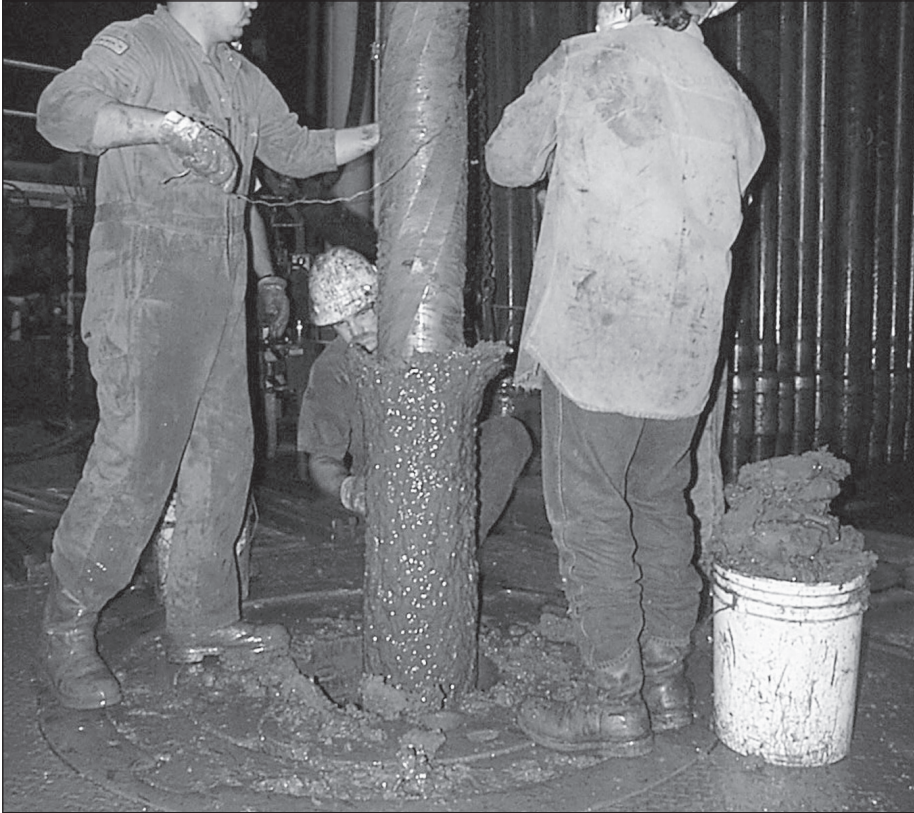
Fig. 13–4. Hydrated clays sticking to a drill collar
