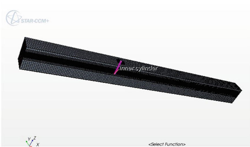
Fig. 5.16 Domain of inner cylinder generated with volumetric control (Chandrasekaran et al. 2014b)
