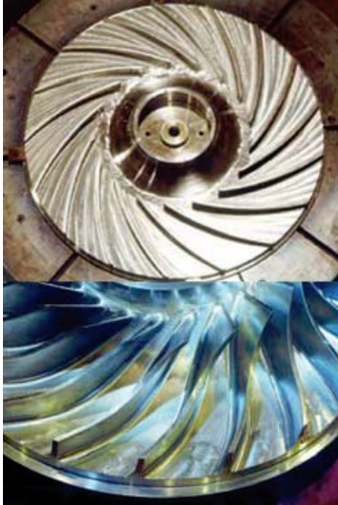
Figure 9.7 2D blades with circular arc shape (top) or 3D blades with complex shape (bottom). Source: From Sorokes (2013), reprinted with permission by AIChE.
