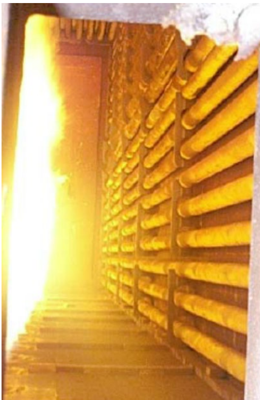
Figure 8.6 An example of flame impingement.
