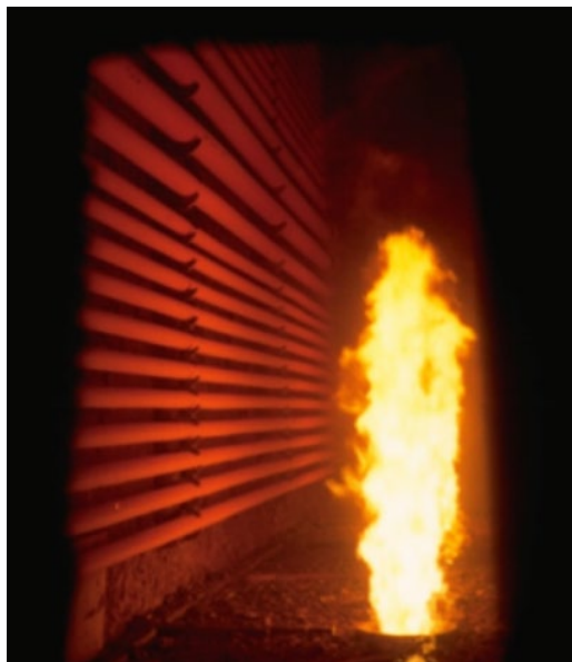
Figure 8.7 Good flame color and height.
