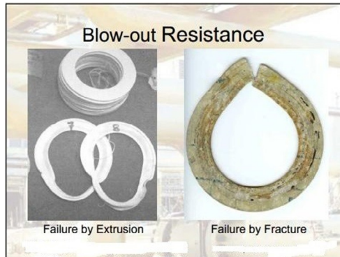
Failure can be by either Extrusion or Fracture
