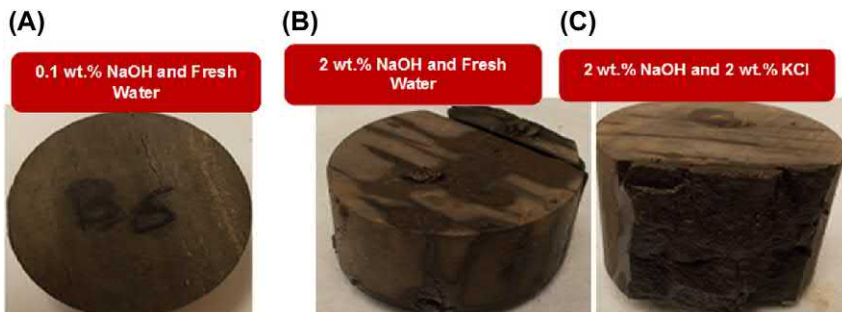
Figure 8.25 Barnett shale samples after being immersed in (A) 0.1 wt% NaOH water, (B) 2 wt.% NaOH water, and (C) 2 wt.% NaOH and 2 wt.% of KCl water.
