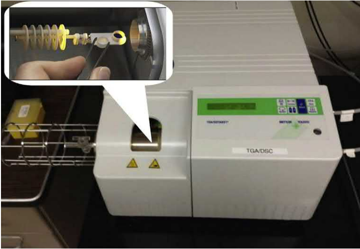
Figure 13.1 An example of TGA apparatus and its sample crucible.
