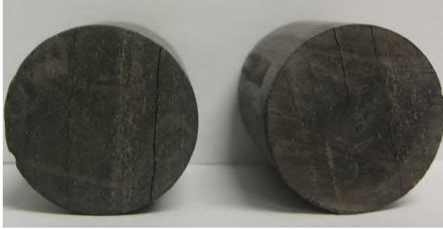
Figure 8.2 Barnett Shale with clear fractures parallel to the bedding after immersion in distilled water.
