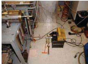
Figure 1.13f. Pump injects oil at constant pressure to simulate reservoir.
