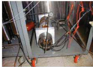
Figure 1.13k. System pump (accumulators are attached to solenoids and powered by system pump).
