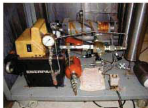
Figure 1.13l. Hydrostatic pump (hydrostatic and formation pressures maintained by accurate, point-operating relief valve attached to formation and hydrostatic pumps).
