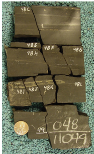
FIGURE 3.23 Upper black shale member of the Bakken Formation in a core slab, showing pyrite laminae, fossil shells, and multiple fractures. Coin for scale is 2 cm in diameter. Photo from North Dakota Geological Survey.
