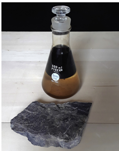
FIGURE 3.19 Crude oil from the Bakken Formation floating on produced water. A hand sample of Bakken-equivalent shale from beneath the Lodgepole limestone is shown in the foreground. Photographed in 2019 by Dan Soeder.
