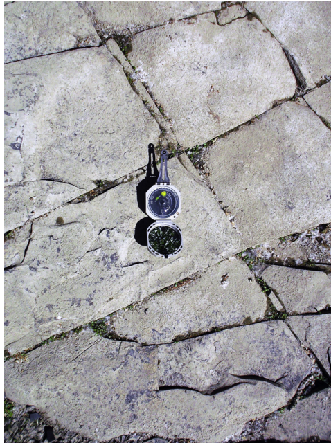
FIGURE 2.11 Orthogonal joints on a flat bedding plane of the Marcellus Shale, exposed in the bed of Oatka Creek, Leroy, NY. The compass points to the north. Photo by Dan Soeder.
