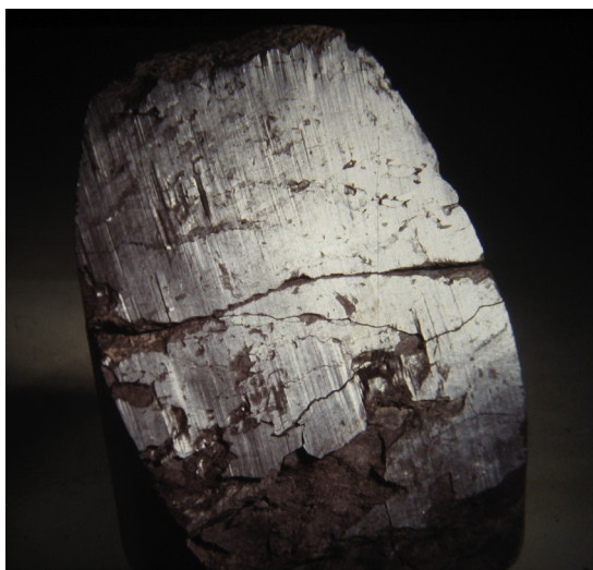
FIGURE 2.10 A slickensided fault surface cutting across a 3.5 inch (9 cm) diameter EGSP shale core. Photo by Dan Soeder.
