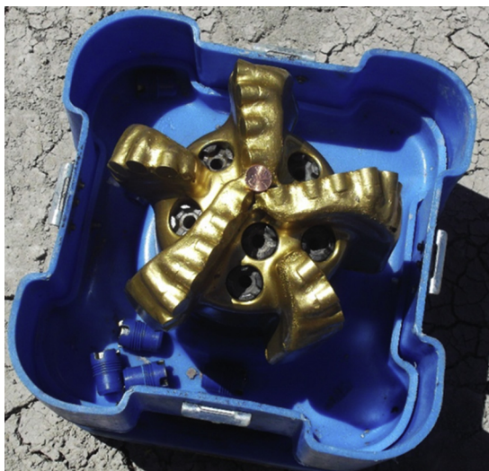
FIGURE 2.7 Polycrystalline diamond composite drill bit used on the Niobrara Formation in the Denver–Julesburg basin, eastern Colorado. Jets in the hub are designed to flush mud off the cutting teeth. Coin in the center for scale is 2 cm in diameter. Photograph by Dan Soeder.
