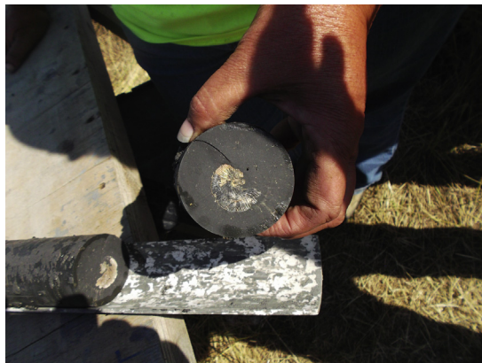
FIGURE 4.8 Organic-rich Pierre Shale drill core from Presho, SD with an ammonite fossil on a parting surface. Photographed in 2015 by Dan Soeder.
