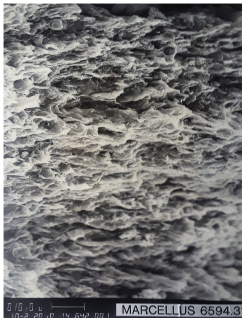
FIGURE 2.4 Scanning electron micrograph of a freshly broken surface on Marcellus Shale perpendicular to bedding. Scale bar is 10 \mu\text{m} . Clay fabric and structure are clearly visible, but the “pores” are actually voids created by the removal of preexisting grains. DOE photo.
