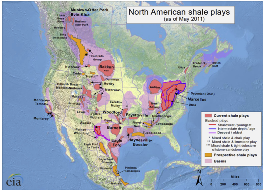
FIGURE 2.9 Shale gas and tight oil plays in North America. Much of the current focus is on stacked plays in the Appalachian, Permian, and Powder River basins and on liquids-rich plays like the Eagle Ford, Bakken, and Utica. Reproduced from U.S. Energy Information Administration reports and web pages.
