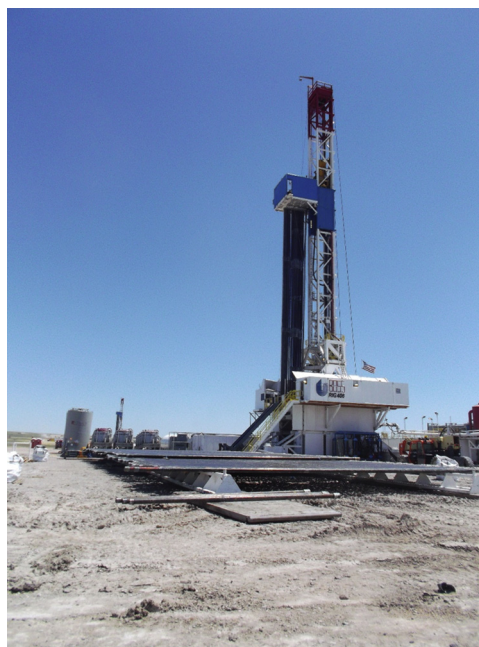
FIGURE 2.6 A large, “triple” hydraulic drill rig installing a lateral into the Niobrara Formation at a depth of approximately 8000 ft (2.4 km) in the Denver–Julesburg basin, eastern Colorado. Scale is indicated by the stairway and entrance door of the “dog house” office trailer attached to the side of the platform and used to operate the rig. A second rig is visible in the background at left. Photo by Dan Soeder.
