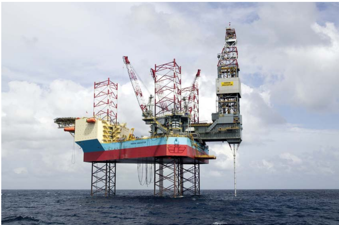
Fig. 1.16—Jackup rig. Courtesy of Maersk Drilling.
