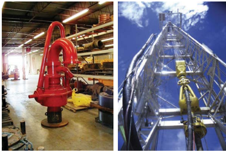
Fig. 1.28—(a) Rotary swivel (Steven M. Hain Company, Inc. 2010); used with permission from Steven M. Hain Company, Inc.; (b) rotary swivel (courtesy of OSHA).
