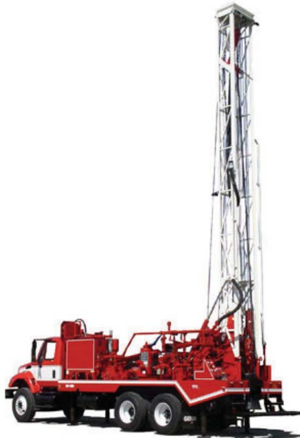
Fig. 1.12 —Mobile rig with portable mast (GEFCO 2007). Courtesy of GEFCO.
