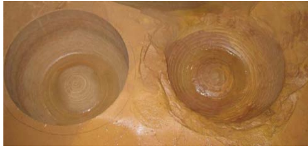
Fig. 6.43a—Stable (left) and unstable (right) PDC at high RPM. Instability caused continuous fracturing (Johnson 2006).
