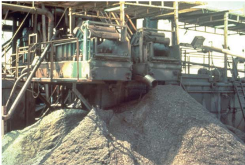
Fig. 3.26—Typical shale shaker [from Oilfield Glossary (2011)]. Courtesy of Mark Ramsey/Texas Drilling Associates.
