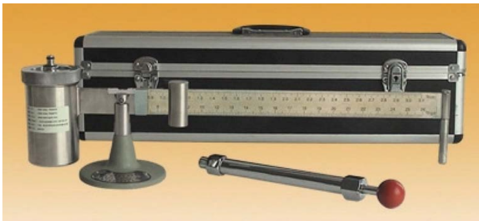
Fig. 4.2—Mud balance. Courtesy of Halliburton.
