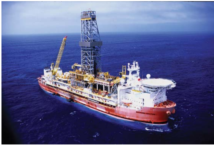
Fig. 1.19—A modern ultradeepwater drillship operating in Campos Basin, Brazil (courtesy of Petrobras SA).
