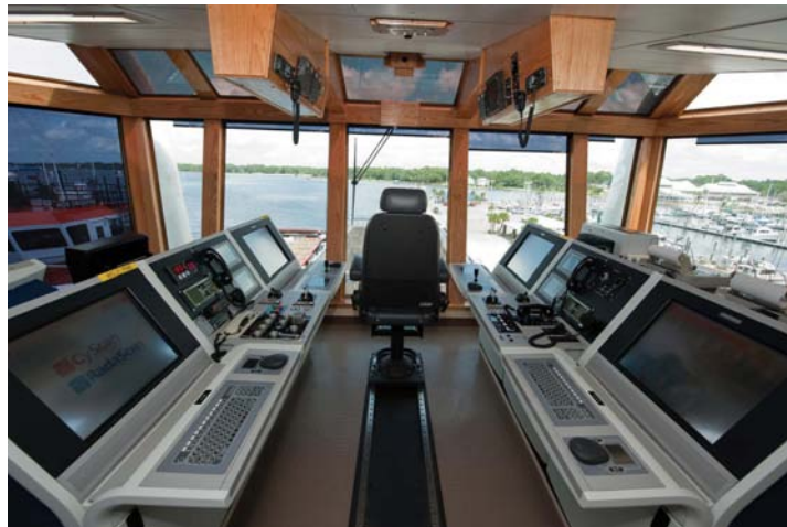
Fig. 1.37—DP control room. Courtesy of Keith Wyatt, Converteam.
