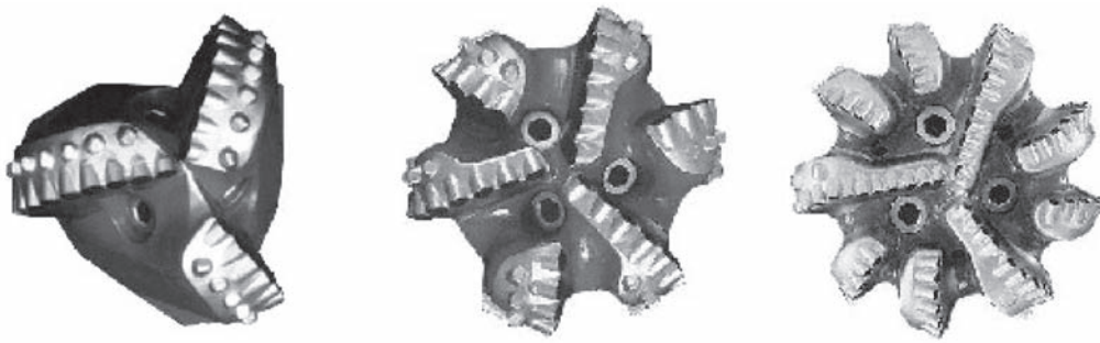
Fig. 6.20—Soft- (left), medium- (middle), and hard- (right) formation blade/cutter combinations for a PDC bit (Chevron DE Drilling Seminar 2005).
