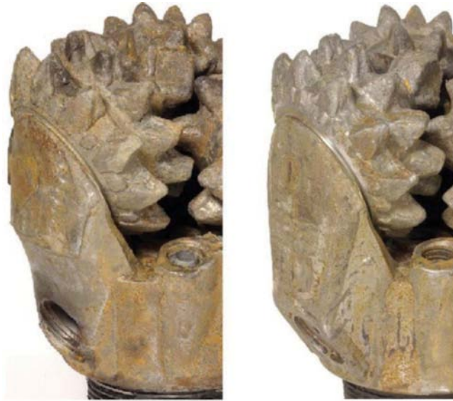
Fig. 6.10—Left = standard hardfacing; right = enhanced hardfacing (Buske et al. 2008).
