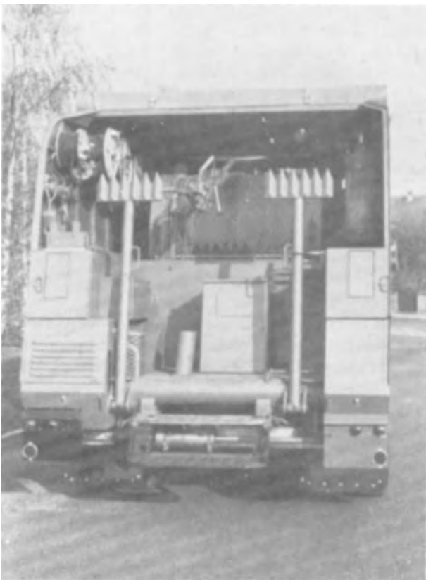
Fig. 2-16. Rear view of a logging truck, showing the cable and spooler (courtesy of Schlumberger).
