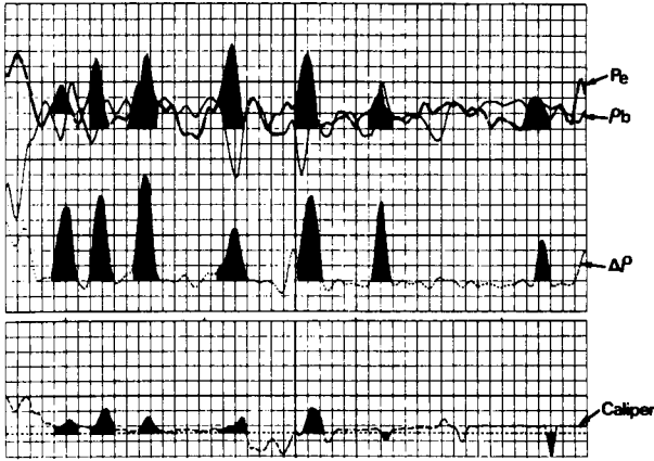
Fig. 12-8. Barite effect on log response. This can be used as fracture detection (courtesy of Schlumberger).
