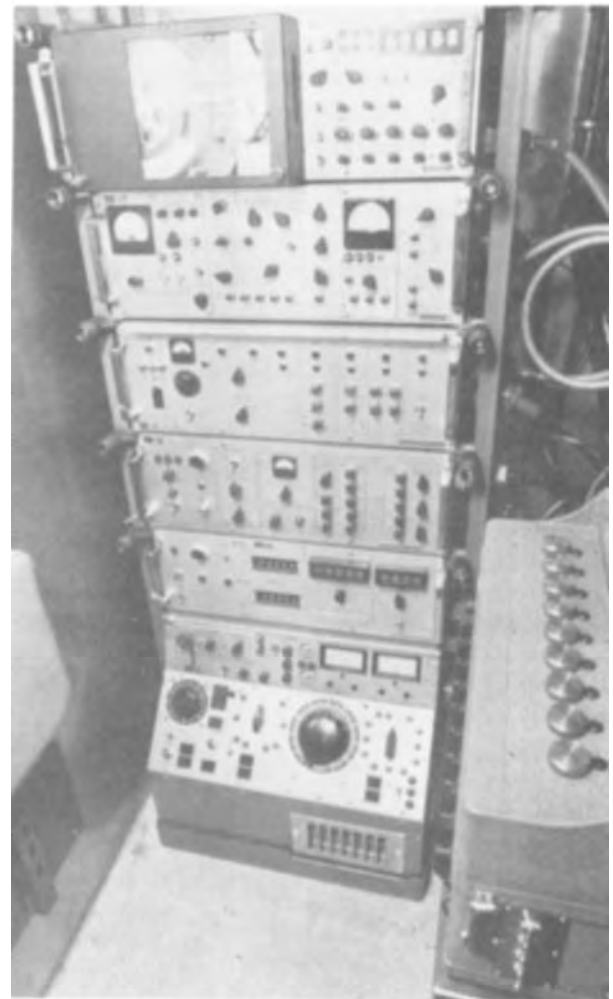
Fig. 2-17. A view inside the truck, showing the logging panels, tape recorder (top) and part of the camera (right) (courtesy of Schlumberger).
