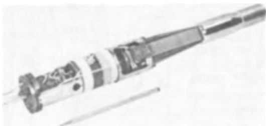
Fig. 10-11. High-voltage stage providing the accelerating voltage for the neutron generator.
