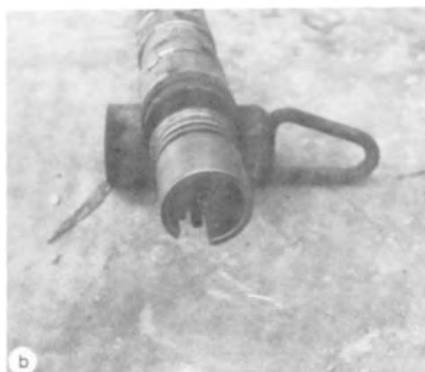
Fig. 2-20. a. The bridle (note the electrodes, head, and part of the quick connection). b. The bridle-head.
