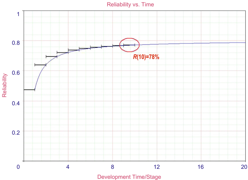
FIGURE 2-24 Reliability \times Time Stages (Lloyd-Lipow model).
