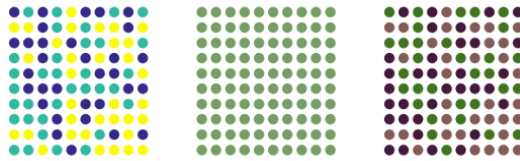
Figure 1.2. Sketch of the separation coherent/incoherent. A single atomic sample with three isotopes (problem reduced to the static part of the isotopes here) is split in its average scattering length \bar{b} on all nuclei plus the fluctuations around the mean value for each nucleus ( b_j^2 - \bar{b}^2 ). For a color version of this figure, see www.iste.co.uk/broseta/hydrates1.zip
