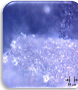
Figure 2.15. Characteristic microscopic view (objective \times 50 ) of the recovered natural gas hydrate. The opaque zones with a rough and irregular surface correspond to the presence of gas hydrate. Light areas (white marks of \sim 10 \mu\text{m} ) correspond to the presence of ice. Adapted with permission from [CHA 04]. For a color version of this figure, see www.iste.co.uk/broseta/hydrates1.zip
