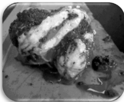
Figure 2.17. Recovered gas hydrate samples from the Nigerian margin. Adapted with permission from [CHA 07]
