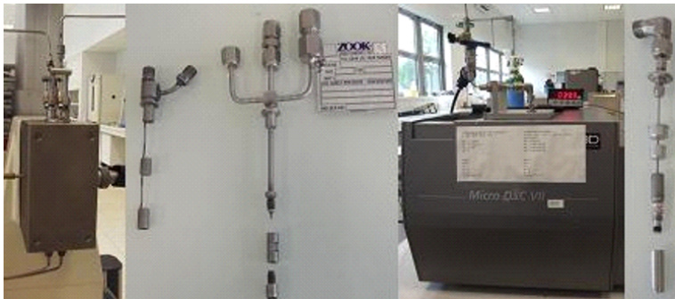
Figure 4.5. Equipment used at ENSTA ParisTech for calorimetric study of gas hydrates. From left to right: furnace of the DSC 111 Tian-Calvet calorimeter (SETARAM); 100 and 400 bar pressure-controlled cells for the DSC 111; \mu\text{DSC VII} calorimeter (SETARAM); pressure-controlled cell for the \mu\text{DSC VII} . For a color version of this figure, see www.iste.co.uk/broseta/hydrates1.zip
