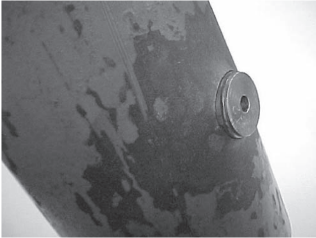
Figure 11-16: A Check Valve and Orifice for Gas Lift Installed in Tubing Using Wireline Techniques
