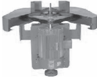
Figure 15-28: Surface PCP Drive Systems
