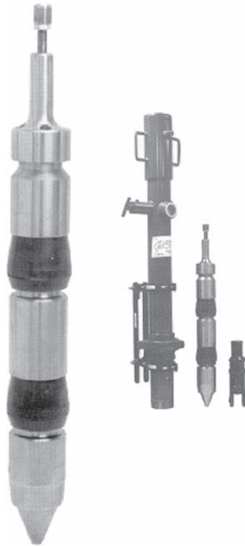
Figure 7-25: Casing Plunger Showing the Rubber Cups That Seal against the Casing ID and the Lubricator and Downhole Casing Stand (Multi Products Co., Millerburg, OH)
