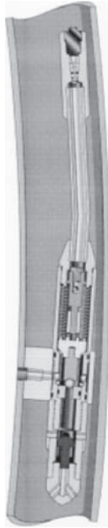
Figure 11-10: Spoolable Coil Tubing Gas Lift System (Schlumberger)
