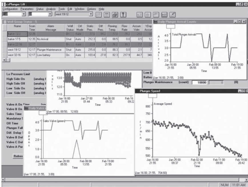
Figure 15-21: Plunger Lift Surveillance Panel
