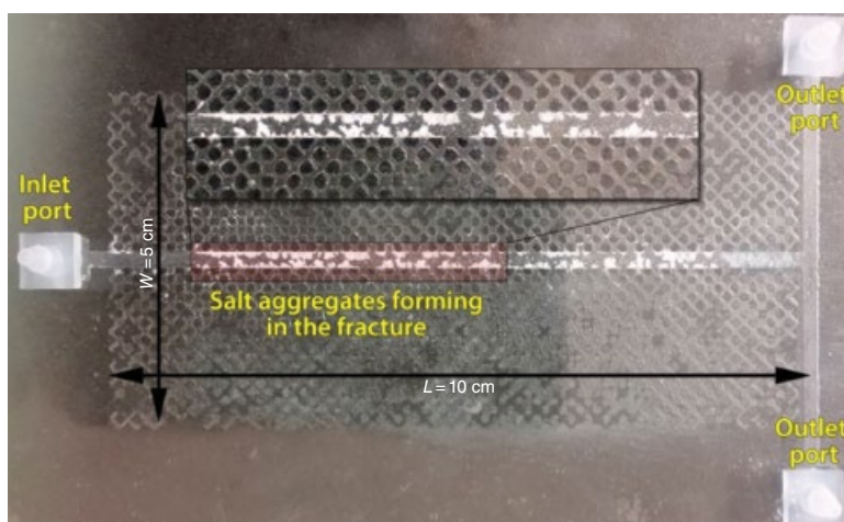
Figure 8.6 Pore-scale visualization of salt precipitation in the preferential pathway (fracture) of the heterogeneous microchip. After Miri et al. [2015]. A thick film of brine remains after CO 2 invasion at 5 s after injection. After 50 min, this film evaporates and the drying front shapes a meniscus at the interface between matrix and fracture. After 75 min, aggregation growth starts and occupies the fractures.
