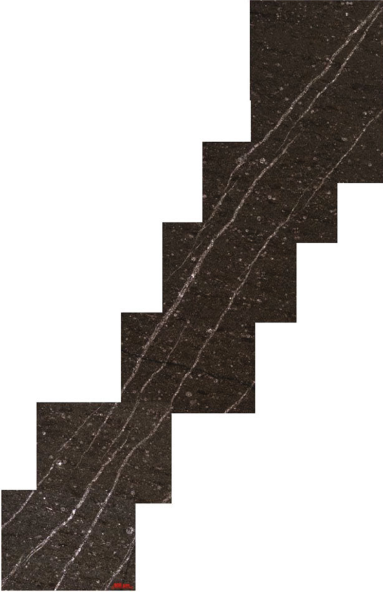
Fig. 6.10 Photomosaic illustrating parallel continued fractures recrystallized by calcite. Taken with crossed Nicols (2.5X)
