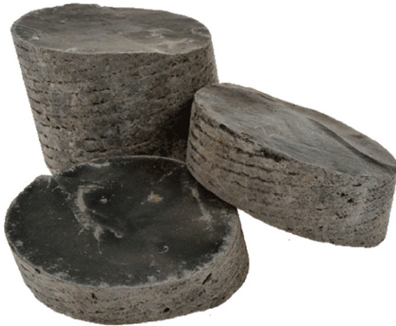
FIGURE 9.2 Core samples from Barnett shale reservoir. Extremely low porosity and permeability.
