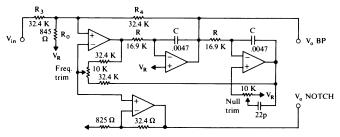
$|A_{VO}|_{NOTCH} < -40 \ dB, \quad Notch \ BW_{-40 \ dB} < 1 \ Hz$
