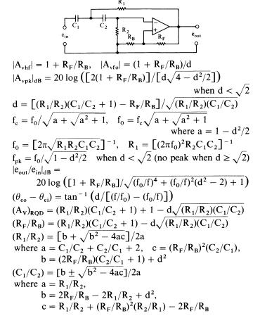
Notes: ① Sallen-Key filters are also known as single feedback, voltage controlled voltage source and VCVS.
