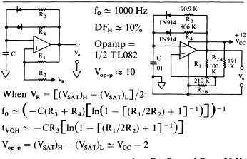
when  $R_3$ ,  $R_4$  and  $R_L > 30 K$
