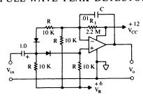
$V_{o(MAX)}$  when  $V_{in} \ge 1V_{p-p}$  sinewave Sensitivity may be decreased by decreasing  $R_1$
