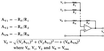
Minimum required peak to peak capability =  $4\sqrt{2} \ V_{0 \, rms(MAX)}$ Input to input isolation =  $20 \log \left[ (A_{VOL}/A_V) R_{in(OPAMP)} \right] dB$  when inputs driven from current source
