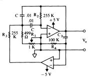
$$f_0 = [2\pi C\sqrt{R_1R_2}]^{-1} \simeq 850 \text{ to } 1350 \text{ Hz}$$
