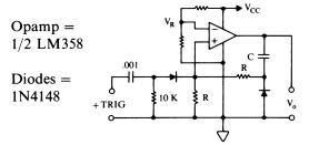
$$\begin{split} t_{on} &= 2RC \big(ln[V_{o(MAX)}/2V_R]\big) \\ &\qquad \qquad (V_{o(MAX)} \simeq V_{CC} - 1.2 \text{ when } I_o \leq 1 \text{ mA}) \\ t_{on} &= 2RC \quad \text{when } V_R = .184V_{o(MAX)} \end{split}$$
