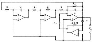
$$f_0 = [2\pi RC]^{-1}, \quad Q = R_0(2\pi f_0 C)$$
