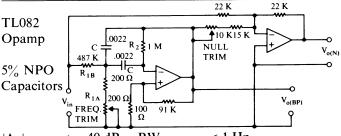
$|A_V|_{NOTCH} < -40 \ dB, \quad BW_{N(-40 \ dB)} < 1 \ Hz$
