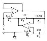
With only a high Q capacitor connected to the L input and R<sub>3</sub> tweaked to the edge of oscillation, circuit Q is very close to infinite.
