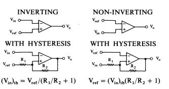
Add diode in series with R<sub>2</sub> for unidirectional hysteresis
