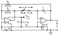
Opamp = TL82 etc(Transpose R3 and R4 when using "single supply" opamps)
