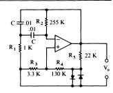
$$f_0 = \left[2\pi C \sqrt{R_1 R_2}\right]^{-1}$$
