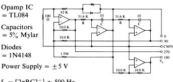
$$f_0 = [2\pi RC]^{-1} \simeq 500 \text{ Hz}$$
