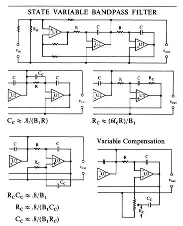
Short  $R_0$  and tweak  $R_C$  or  $C_C$  to the edge of oscillation for best general formula accuracy. This also compensates for capacitor Q.
