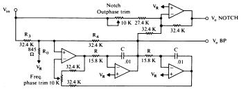
$|A_V|_{NOTCH} < -40 \ dB, \quad (BW_N)_{-40 \ dB} < .5 \ Hz$
