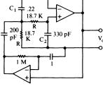
$f_0 \simeq [2\pi RC]^{-1}$ \(\sim 1000 Hz\)
