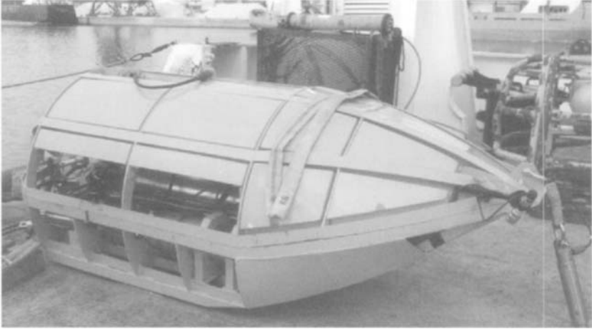
Figure 16.15 GAMBAS® seismic refraction system – seabed tow sled
