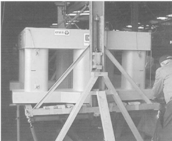
Figure 13.7 Setup of the model on calibration table (Courtesy of Offshore Model Basin)
