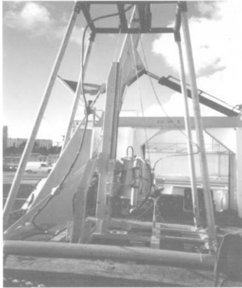
Figure 16.37 Example of seabed mounted rock corer – the Sorotel rock corer
