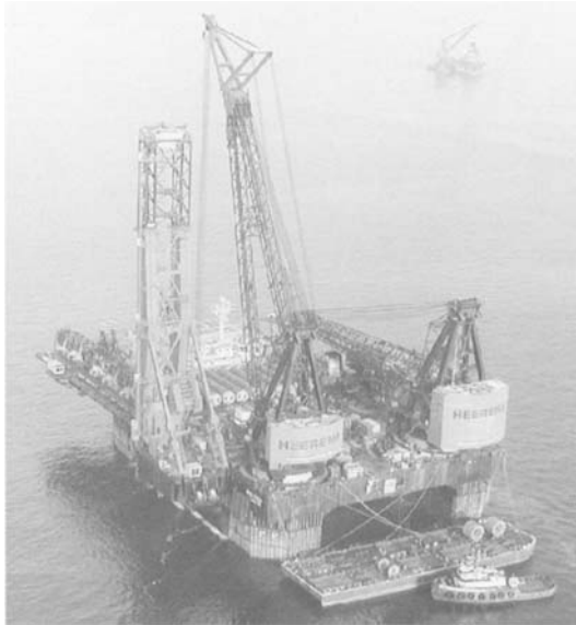
Figure 11.16 Heerema's balder in J-lay mode – Courtesy Heerema marine contractors
