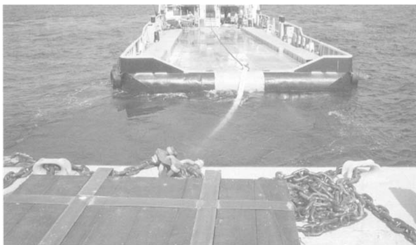
Figure 14.23 Typical arrangement of tow line and bridle
