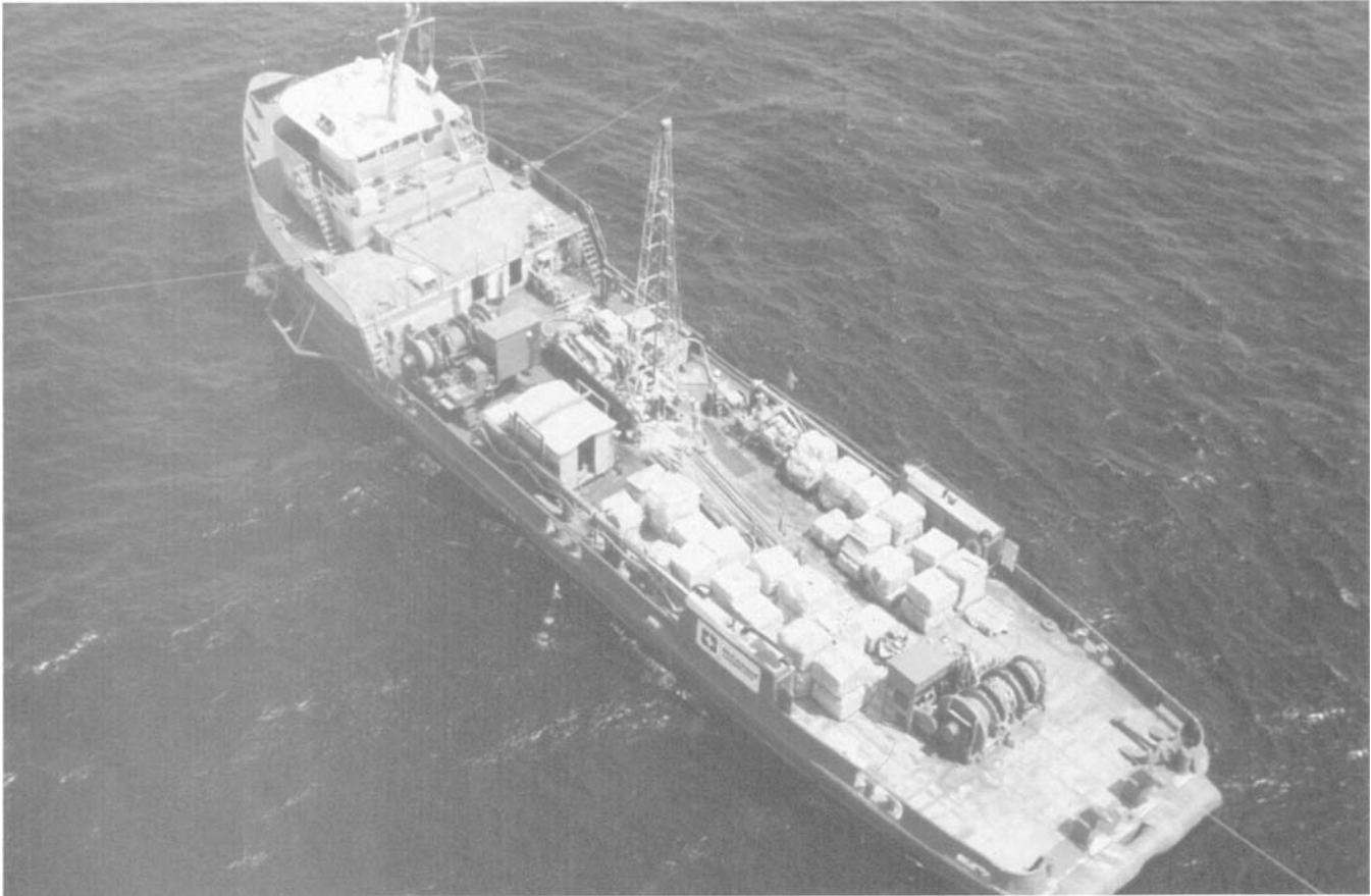
Figure 16.19 Typical supply vessel with skid mounted drill rig – M/V Perkins
