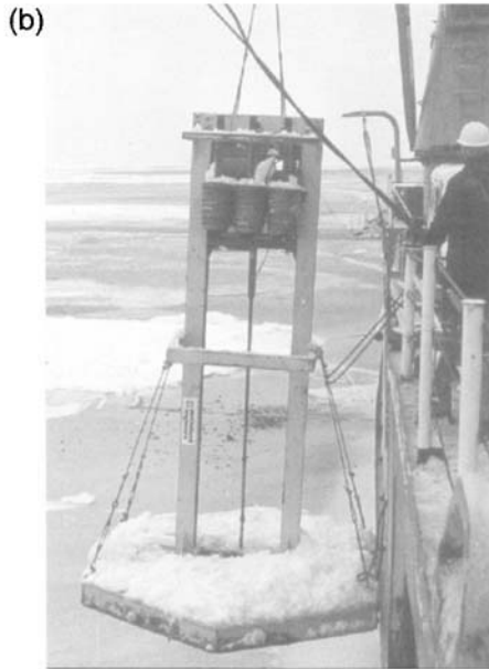
Figure 16.49 (a) SEAROBIN CPT and schematic; (b) Starfish CPT
