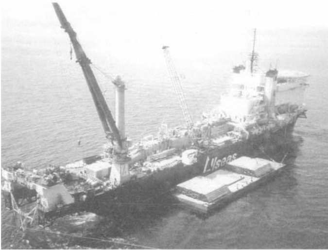
Figure 11.17 Allseas Lorelay S-lay vessel – Courtesy C. Langner
