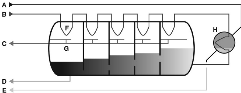
Figure 8.3 Schematic of a multistage flash desalinator.
