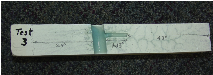
FIGURE 14.37 Smaller hole caused creation of the fracture in both sides.
