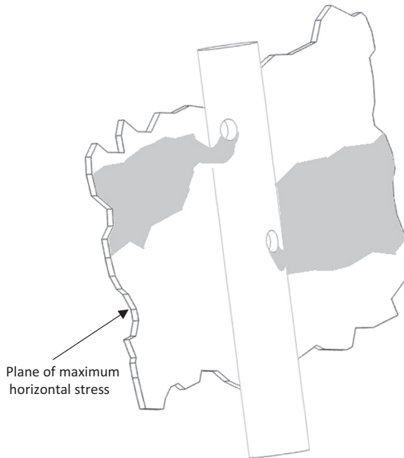
FIGURE 13.1 Schematic showing fractures (gray) exiting the perforations of a wellbore and twisting around the wellbore to eventually propagate in the direction of maximum horizontal stress (perpendicular to minimum horizontal stress). This twisting behavior and the associated pressure drop is one example of near-wellbore tortuosity behavior.
