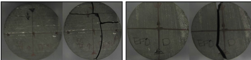
FIGURE 10.2 Tensile failure of an Eagle Ford shale sample with horizontal (left) and vertical (right) laminations ( Mokhtari and Tutuncu, 2016 ).
