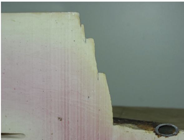
FIGURE 14.29 Cross-sectional view of the oblique wellbore, showing multiple fractures.
