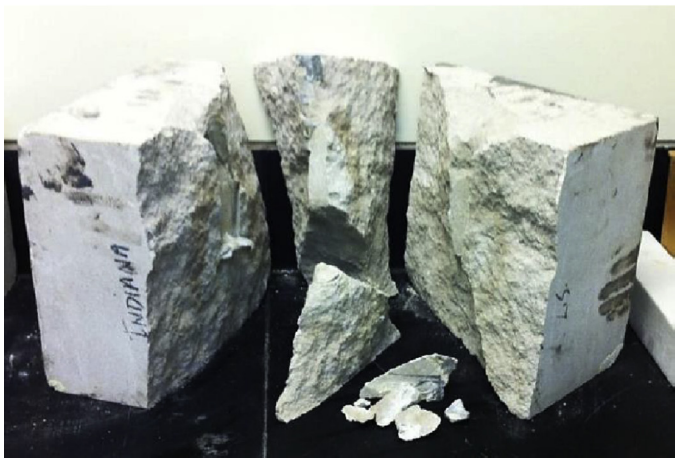
FIGURE 14.64 Indiana Limestone block before (top) and after (bottom) applying fracturing technique using chemically pulsed pressure.
