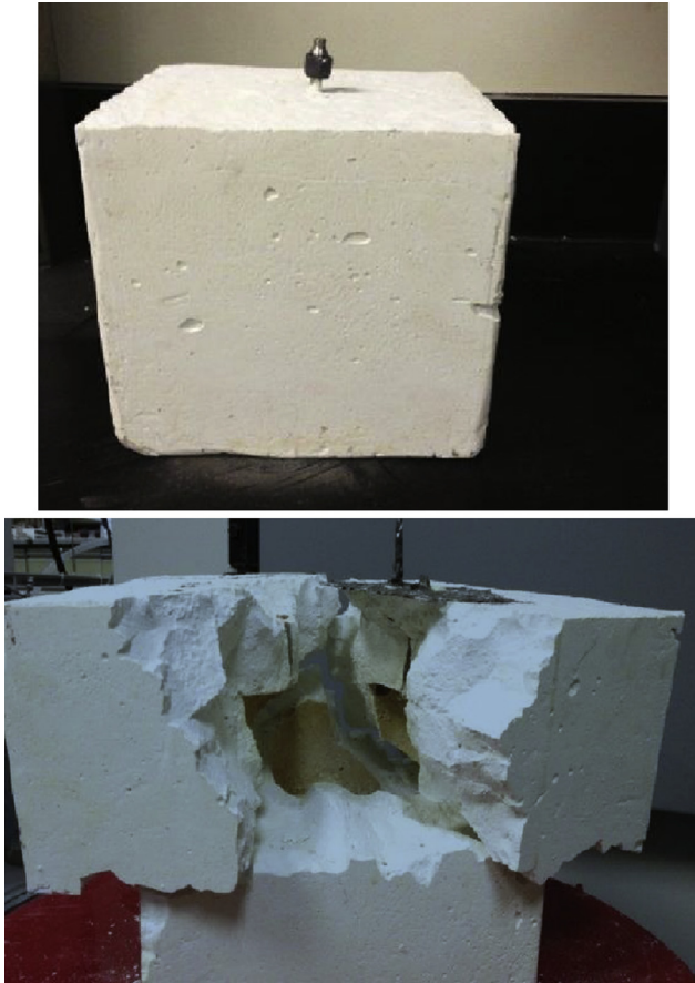
FIGURE 14.63 White cement block before (top) and after (bottom) applying fracturing technique using chemically pulsed pressure.
