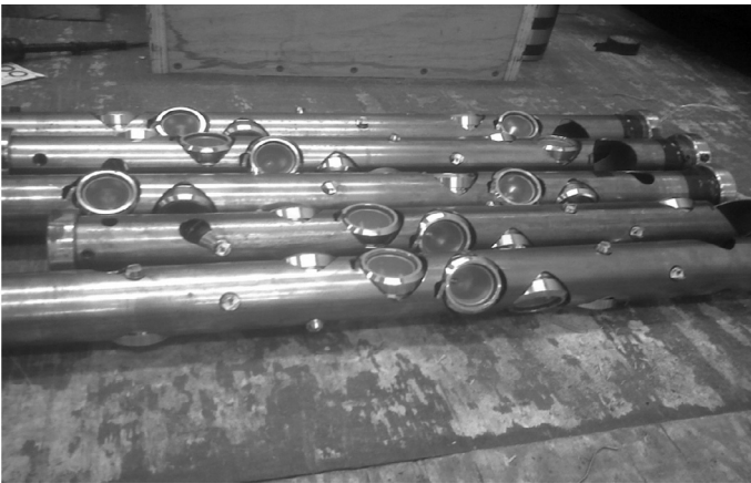
Fig. 11.3 Inside view of perforation guns.
