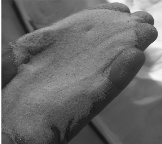
Fig. 6.4 100 mesh sand size.
