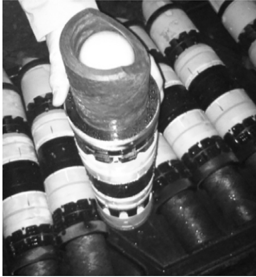
Fig. 11.4 Frac ball inside of a composite bridge plug for frac stage isolation.
