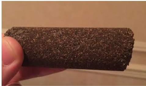
Figure 6.2 Curable resin-coated proppant under reservoir conditions.
