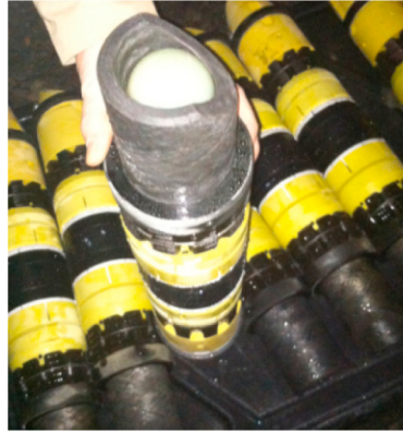
Figure 11.4 Frac ball inside of a composite bridge plug for frac stage isolation.
