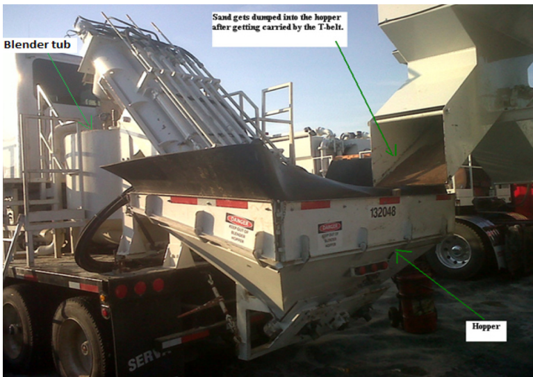
Figure 16.7 Hopper and blender screws.
