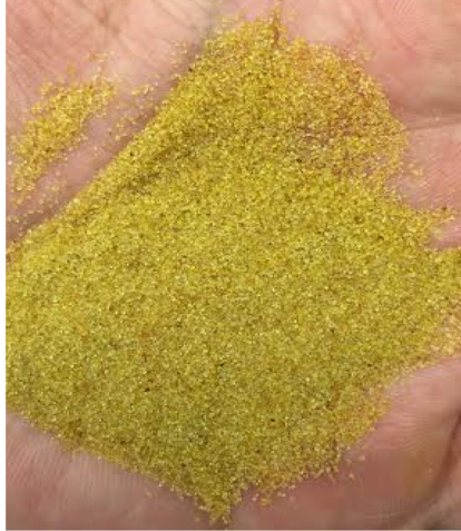
Figure 6.1 Curable resin-coated proppant at standard conditions.
