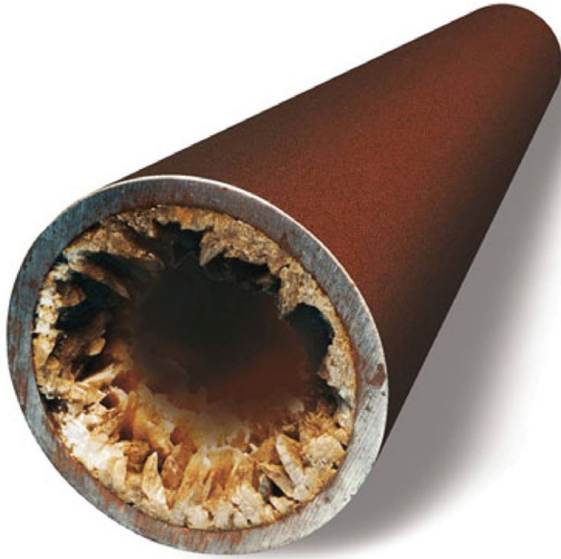
■ FIG. 5.8 Scale accumulations inside tubing. (Courtesy of Schlumberger.)
