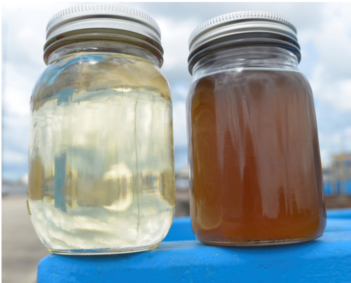
■ FIG. 3.24 Comparison of fresh versus used hydraulic fluid. (Courtesy of Cased Hole Well Service.)
