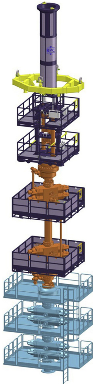
■ FIG. 1.15 Concentric snubbing unit. (Courtesy of Balance Point Control.)
