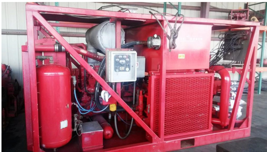
■ FIG. 3.19 Diesel engine-driven power-pack. (Courtesy of Halliburton.)
