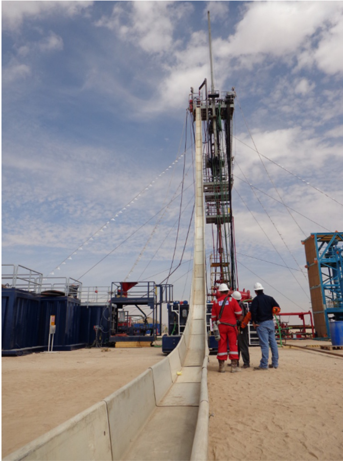
■ FIG. 3.40 Escape slide. (Courtesy of International Snubbing Services.)
