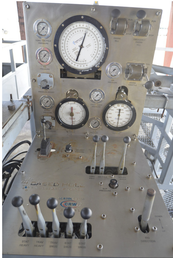
■ FIG. 3.28 Snubbing unit control panel. (Courtesy of Cased Hole Well Services.)
