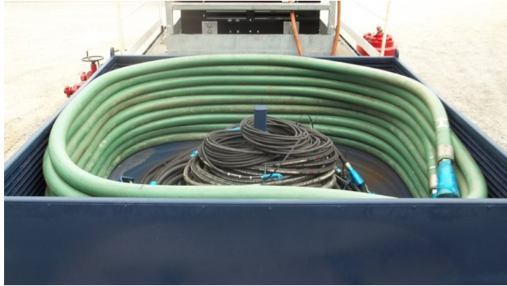
■ FIG. 3.25 Hose basket. (Courtesy of International Snubbing Services.)
