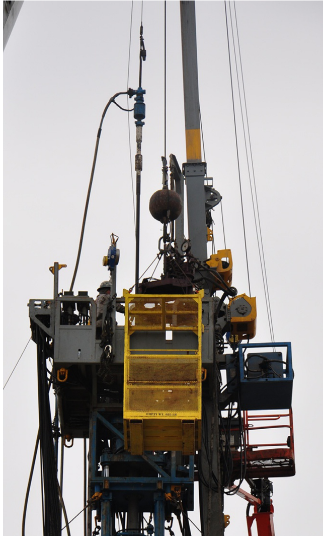
■ FIG. 6.1 Drill string swivel and kelly hose. (Courtesy of Cased Hole Well Service.)
