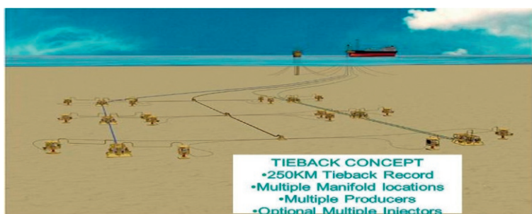
FIGURE 7.2 Example Illustration of Subsea Tiebacks (Source: http://www.intelligent-flow.com ).
