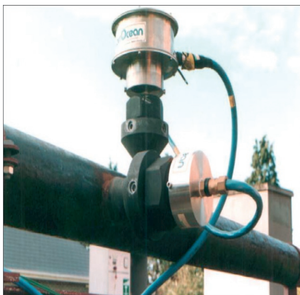
FIGURE 5.8 On-line Intrusive Detector Shown Mounted on a Horizontal Length of Pipe.
