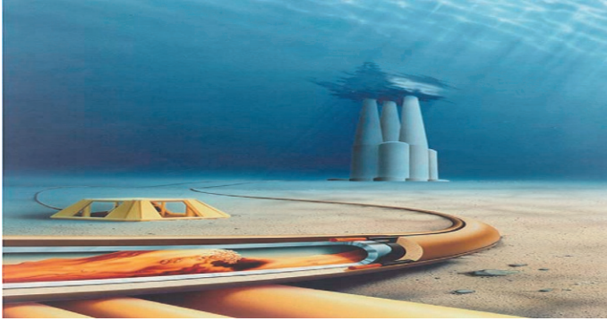
FIGURE 7.3 Subsea Tieback Showing Solids Settling – A Flow Assurance Issue (Source: Bello 24 ).
