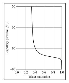
FIGURE 5.3 Relationship between capillary pressure and saturation.
