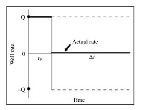
FIGURE 12.2 Rates for the PBU test.
