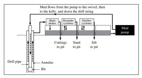
FIGURE 8.8 Illustration of the circulation system.
