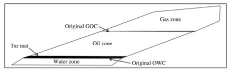
FIGURE 14.6 Schematic cross section of the Prudhoe Bay Field, Alaska.
