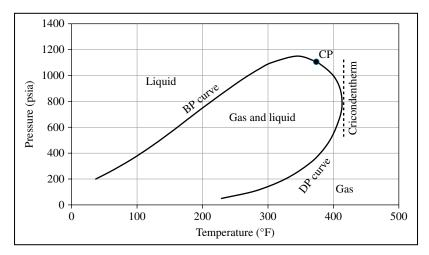
**FIGURE 3.3** Additional nomenclature for P-T diagrams using data for 59/41 mol% ethane/*n*-heptane.
