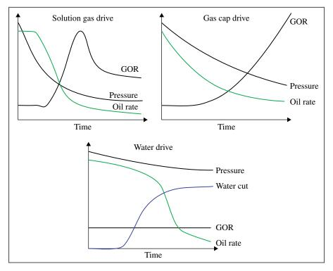
FIGURE 13.3 Production profiles of drive mechanisms.
