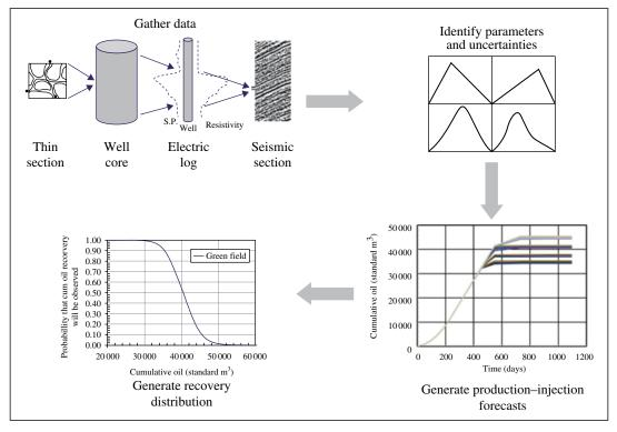
FIGURE 14.2 Green field flow modeling workflow.
