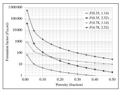
FIGURE 9.7 Sketch of formation resistivity factor for sands.
