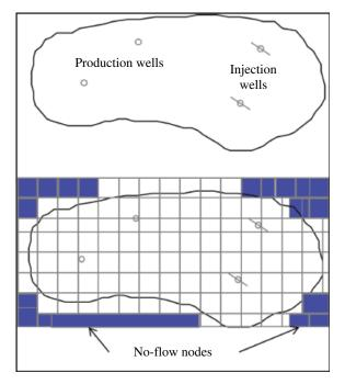
FIGURE 14.1 Overlay of a reservoir grid.
