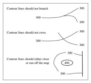
FIGURE 6.8 Examples of contour tips.
