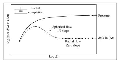
FIGURE 12.5 Log-log diagnostic plot of partially completed well.
