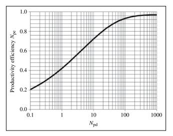
FIGURE 10.1 Brooks' correlation for productivity efficiency of perforations.
