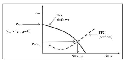
FIGURE 13.5 Illustration of an IPR versus TPC plot.
