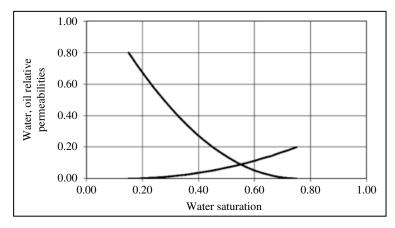
**FIGURE 5.5** Example of water and oil relative permeabilities for a porous medium containing water and oil.
