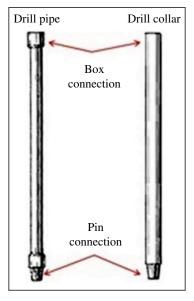
FIGURE 8.6 Drill pipe and drill collar.
