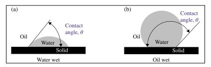
**FIGURE 5.1** Wettability of a surface in contact with two phases is measured by the contact angle.
