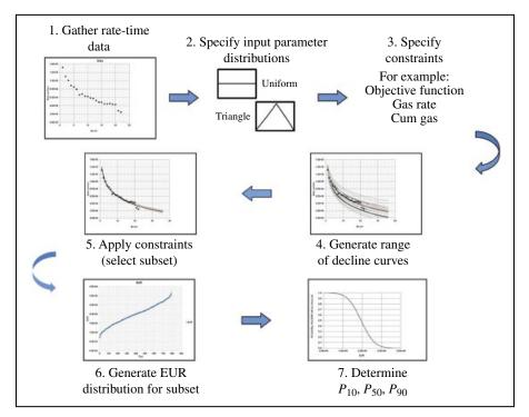
FIGURE 13.2 Probabilistic DCA workflow.
