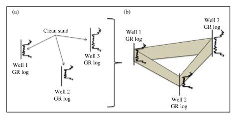
**FIGURE 9.8** Illustration of a fence diagram showing correlation of a clean sand interval. (a) The clean sand interval is indicated by the GR logs. (b) Fence diagram displaying clean sand correlation.
