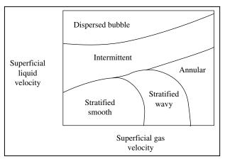
FIGURE 11.8 Illustration of a flow pattern map. (Source: Brill and Arirachakaran (1992).)
