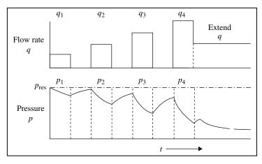
FIGURE 12.9 Modified isochronal test.
