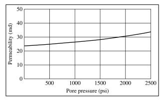
FIGURE 4.3 Pressure dependence of permeability.
