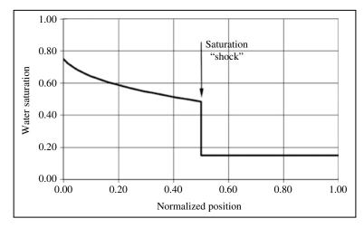
FIGURE 5.11 Water saturation profile when the front is halfway through the sample.
