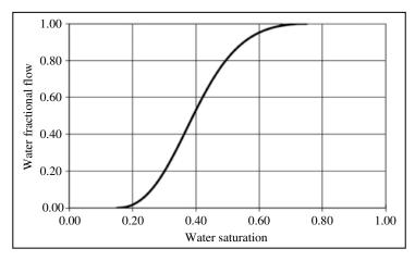
**FIGURE 5.6** Fractional flow for oil–water displacement with relative permeabilities shown in Figure 5.5.
