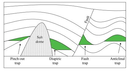
FIGURE 6.9 Examples of traps.
