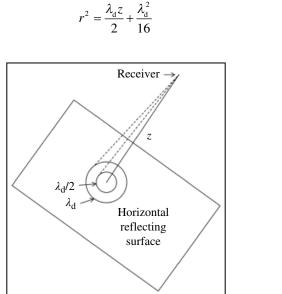
FIGURE 7.5 Geometry of Fresnel zone.
