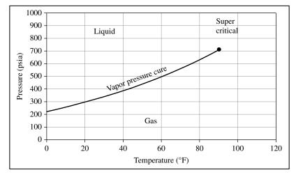
**FIGURE 3.1** *P*–*T* diagram for ethane.
