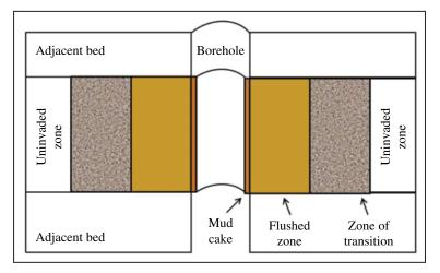
FIGURE 9.2 Schematic of invasion zones.
