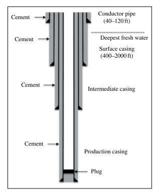
FIGURE 8.10 A wellbore diagram for a vertical well.
