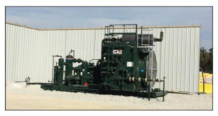
FIGURE 15.2 Gas compressor. (Source: © energy.fanchi.com (2015).)
