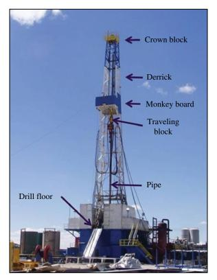
FIGURE 8.1 Modern drilling rig.
