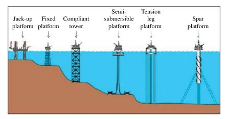
FIGURE 11.10 Examples of offshore platforms.
