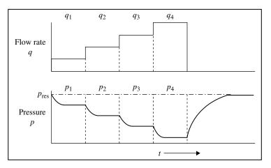
FIGURE 12.7 Conventional backpressure test.
