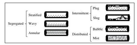
FIGURE 11.7 Flow regimes for horizontal two-phase flow. (Source: Brill and Mukherjee (1999).)
