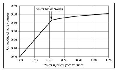
FIGURE 5.10 Oil production during water-oil displacement.
