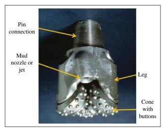
FIGURE 8.7 Roller-cone or tricone drill bit.
