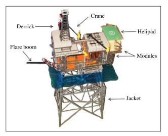
FIGURE 11.12 Key components of an offshore platform.
