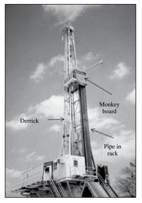
FIGURE 8.3 Derrick with pipe in rack.
