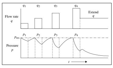
FIGURE 12.8 Isochronal test.
