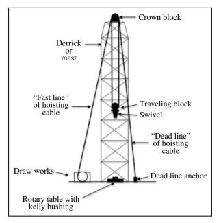
FIGURE 8.2 Illustration of the hoisting system.
