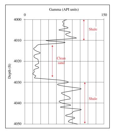
**FIGURE 9.4** Illustration of gamma-ray (GR) log response. Compare with the porosity logs in Figure 9.5 and the resistivity logs in Figure 9.6.
