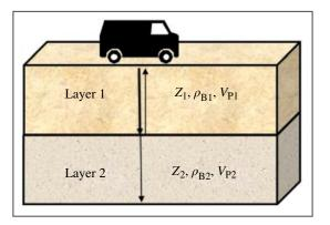
FIGURE 7.4 Seismic attributes for reflection coefficient.
