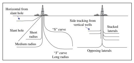
FIGURE 8.12 Directional wells and multilateral wells.
