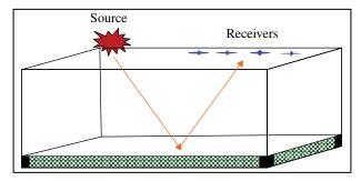
FIGURE 7.1 Energy propagation as vibrations in the subsurface.
