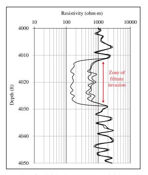
**FIGURE 9.6** Illustration of resistivity log. The three resistivity traces are for shallow, medium, and deep resistivity measurements. Compare with the GR log in Figure 9.4 and the porosity logs in Figure 9.5.
