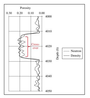
**FIGURE 9.5** Illustration of crossover of porosities from density and neutron logs. Compare with the GR log in Figure 9.4 and the resistivity logs in Figure 9.6.
