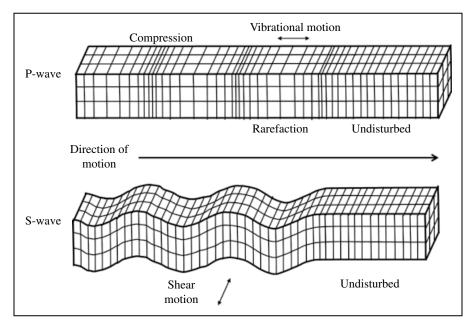
FIGURE 7.2 P-wave and S-wave.
