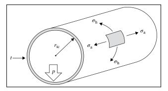
FIGURE 11.4 Stresses on a thin-walled cylindrical pressure vessel.
